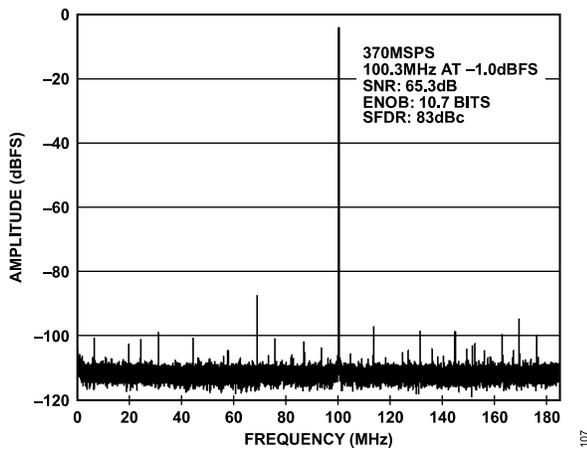
Figure 7. AD9434-370 64k Point Single-Tone FFT; 370 MSPS, 100.3 MHz
