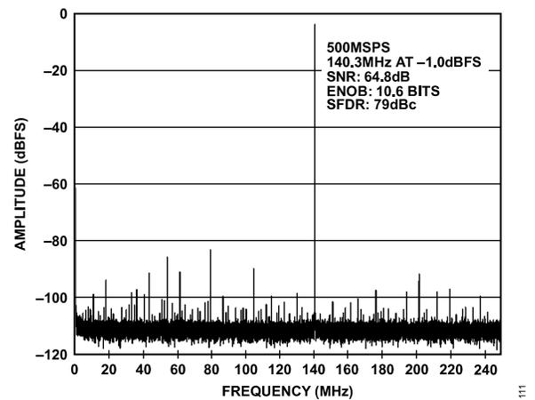
Figure 11. AD9434-500 64k Point Single-Tone FFT; 500 MSPS, 140.3 MHz
