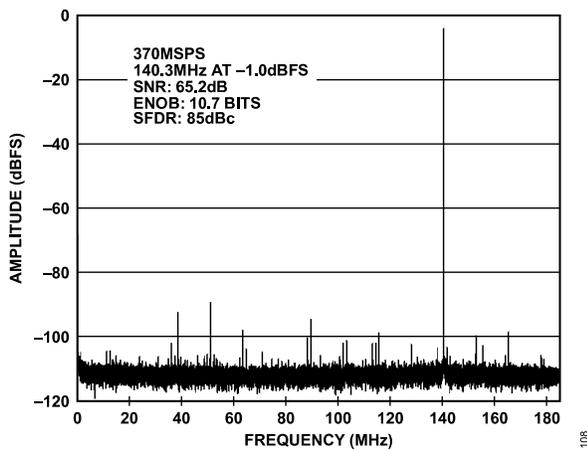
Figure 8. AD9434-370 64k Point Single-Tone FFT; 370 MSPS, 140.3 MHz
