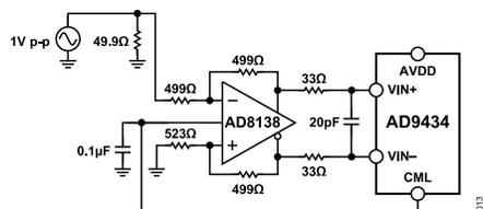
Figure 41. Differential Input Configuration Using the AD8138
