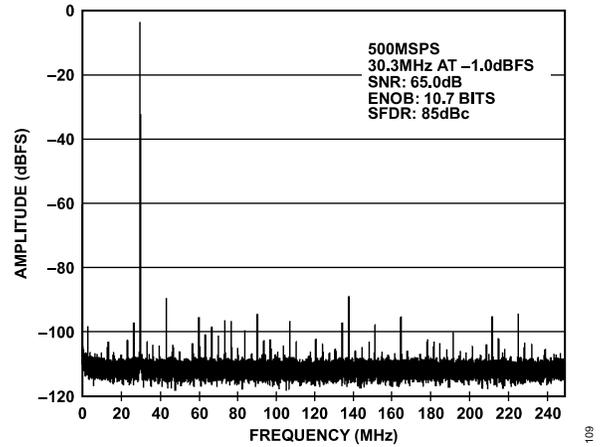
Figure 9. AD9434-500 64k Point Single-Tone FFT; 500 MSPS, 30.3 MHz
