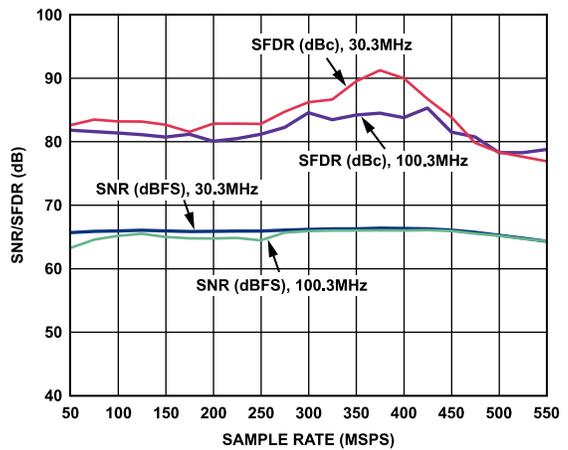
Figure 16. AD9434-370 SNR/SFDR vs. Sample Rate; 30.3 MHz, 100.3 MHz
