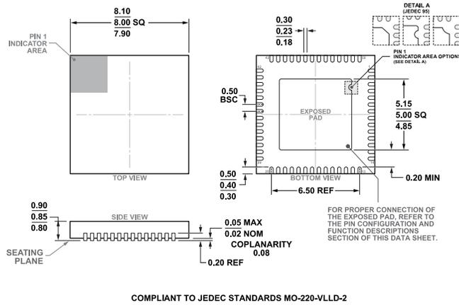
**Figure 53. 56-Lead Lead Frame Chip Scale Package [LFCSP]
