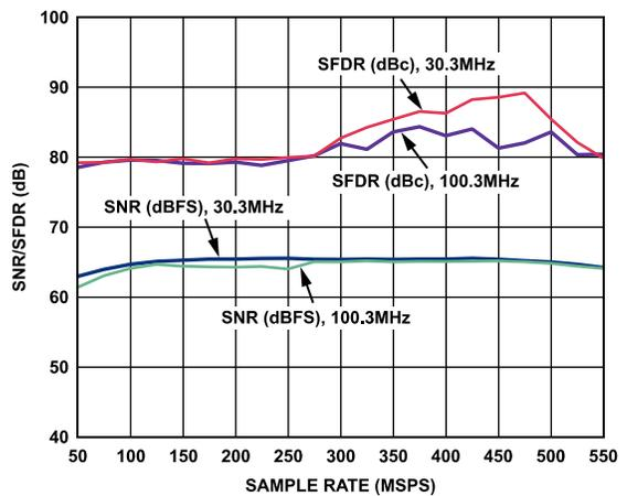
Figure 17. AD9434-500 SNR/SFDR vs. Sample Rate; 30.3 MHz, 100.3 MHz
