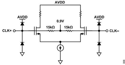
Figure 33. Clock Inputs
