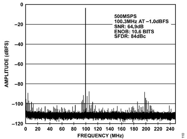
Figure 10. AD9434-500 64k Point Single-Tone FFT; 500 MSPS, 100.3 MHz
