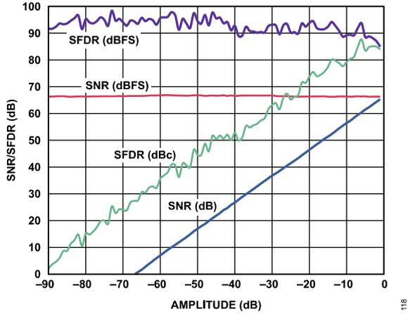
Figure 18. AD9434-370 SNR/SFDR vs. Input Amplitude; 500 MSPS, 140.3 MHz
