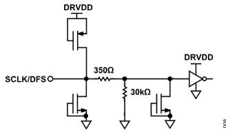
Figure 35. Equivalent SCLK/DFS, PDWN Input Circuit
