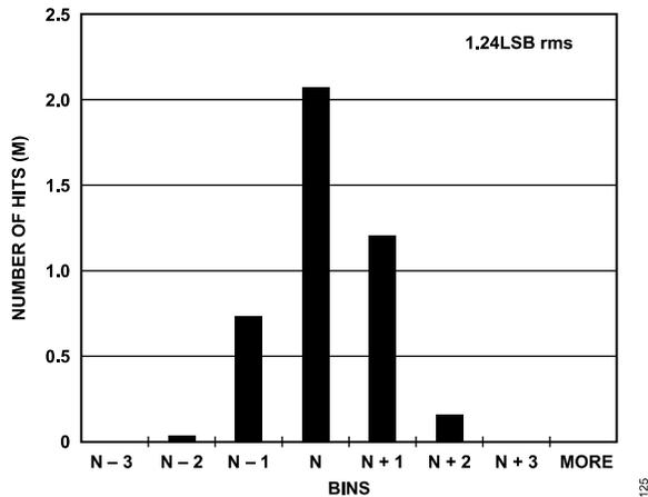
Figure 25. AD9434-500 Grounded Input Histogram; 500 MSPS
