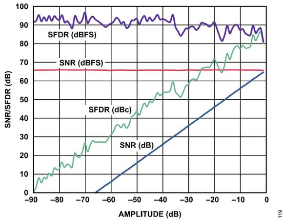
Figure 19. AD9434-500 SNR/SFDR vs. Input Amplitude; 500 MSPS, 140.3 MHz
