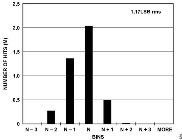
Figure 24. AD9434-370 Grounded Input Histogram; 370 MSPS
