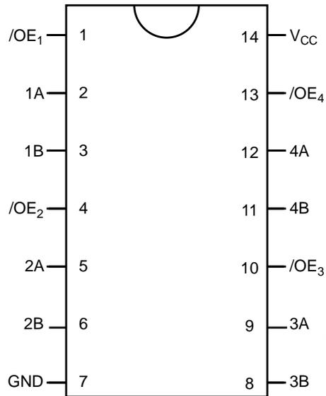
Figure 2. Pin Assignments
