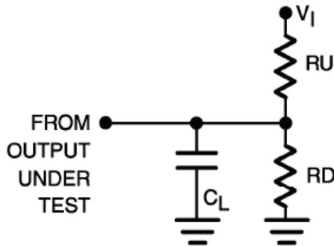
**Notes:** Input driven by  $50\Omega$  source terminated in  $50\Omega$ .
