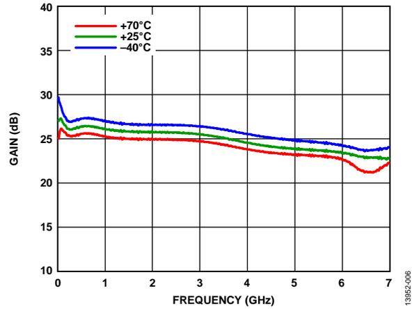
Figure 6. Gain vs. Frequency for Various Temperatures
