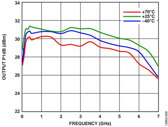
Figure 9. Output P1dB vs. Frequency for Various Temperatures
