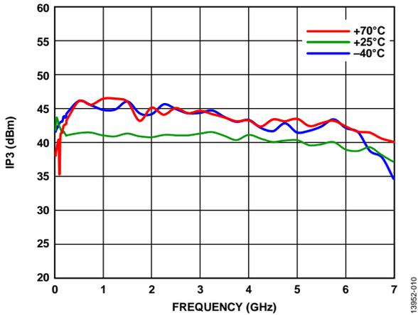
Figure 10. IP3 vs. Frequency for Various Temperatures
