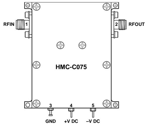
Figure 2. Pin Configuration
