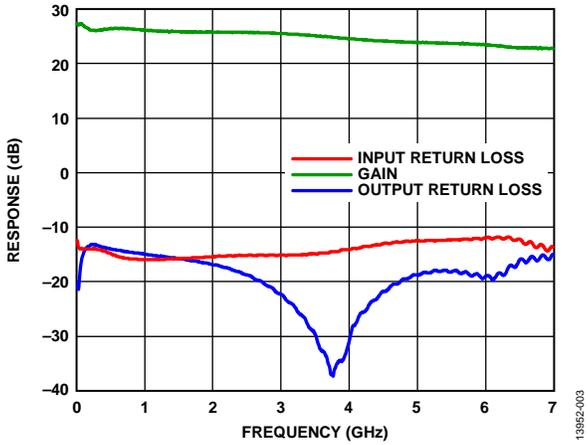
Figure 3. Gain and Input/Output Return Loss vs. Frequency
