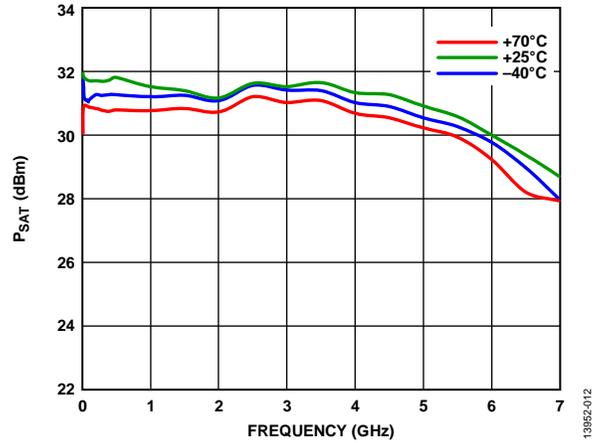
Figure 12. Psat vs. Frequency for Various Temperatures
