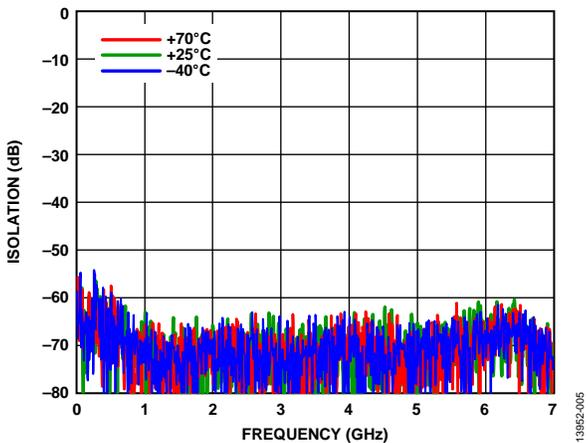
Figure 5. Isolation vs. Frequency for Various Temperatures
