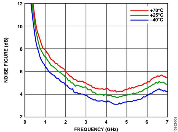
Figure 8. Noise Figure vs. Frequency for Various Temperatures
