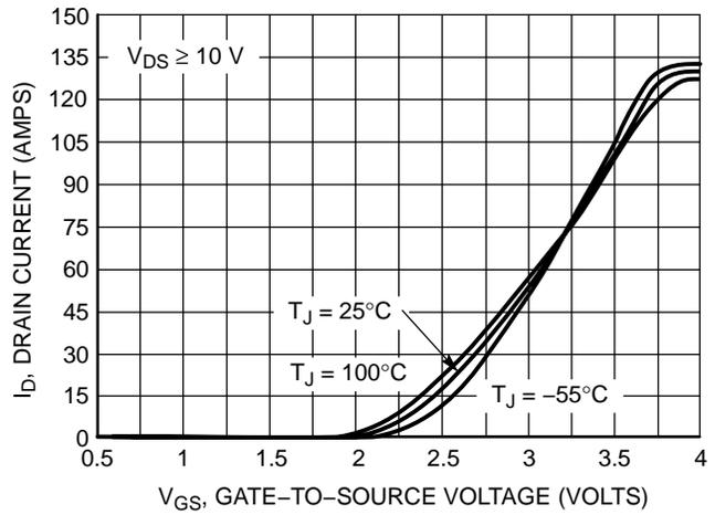
Figure 2. Transfer Characteristics
