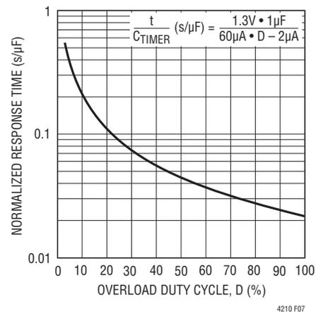
Figure 7. Circuit Breaker Timer Response for Intermittent Overload
