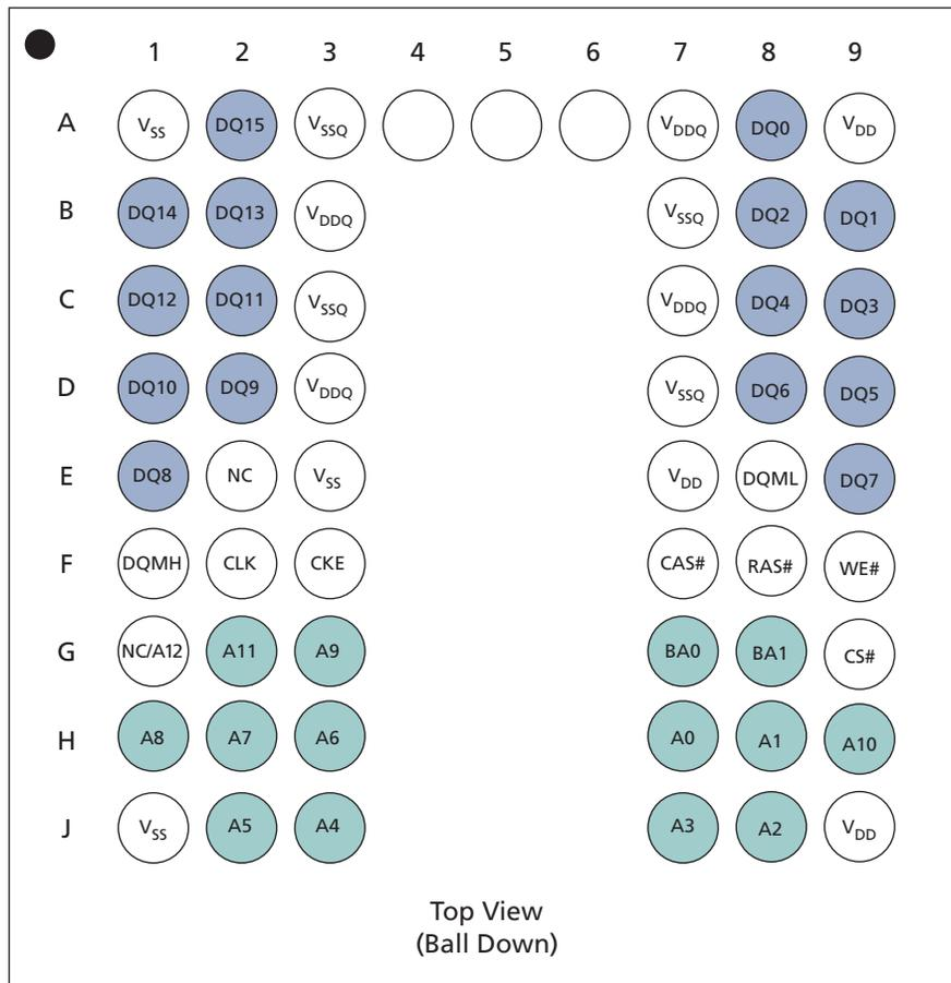
Note: 1. The balls at A4, A5, and A6 are absent from the physical package. They are included to illustrate that rows 4, 5, and 6 exist, but contain no solder balls.
