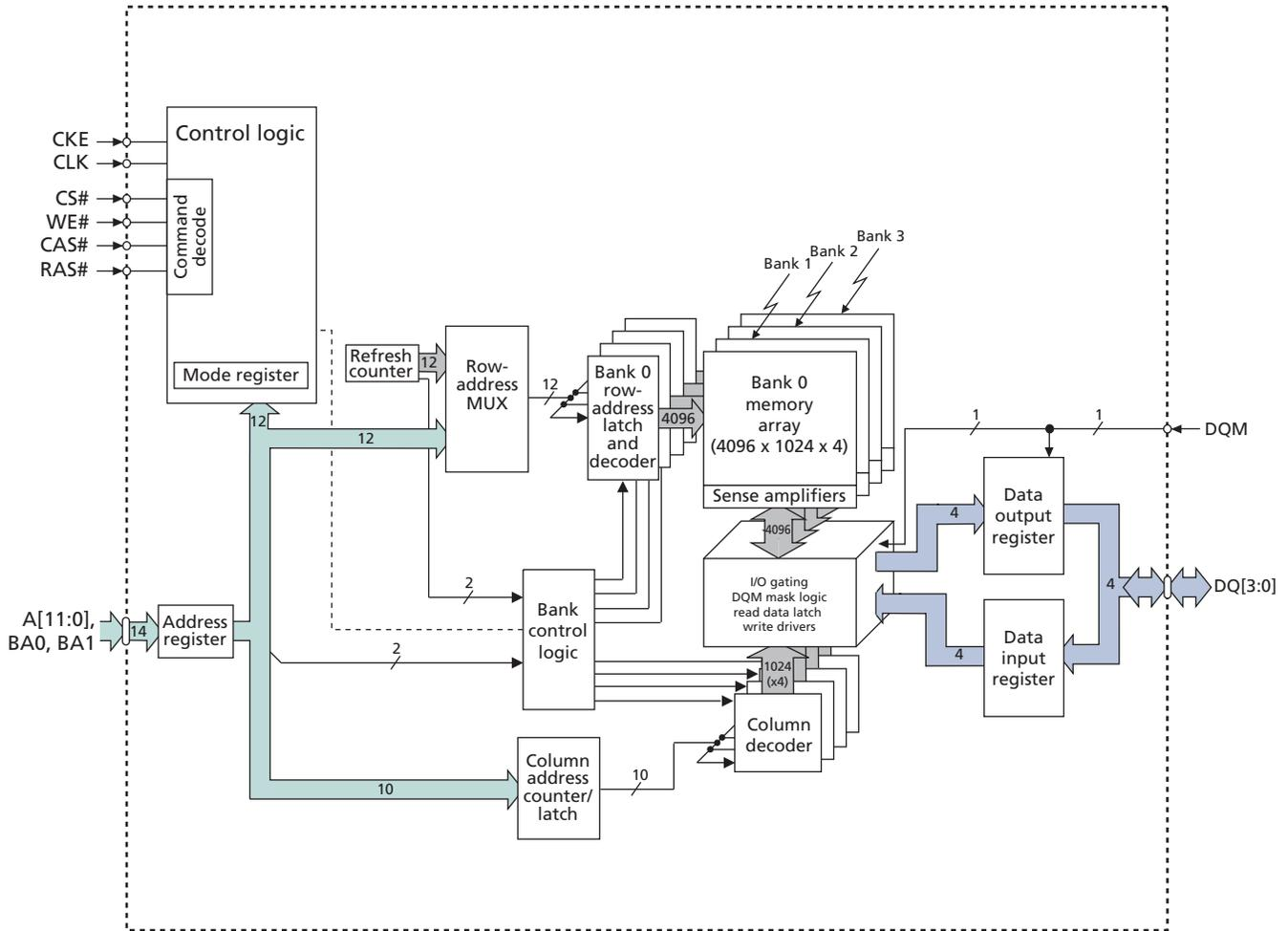
Figure 2: 8 Meg x 8 Functional Block Diagram
