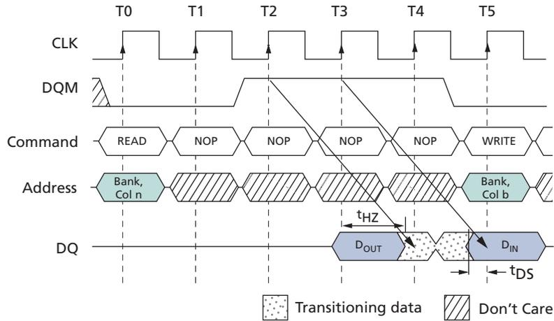
Note: 1. CL = 3. The READ command can be issued to any bank, and the WRITE command can be to any bank.
