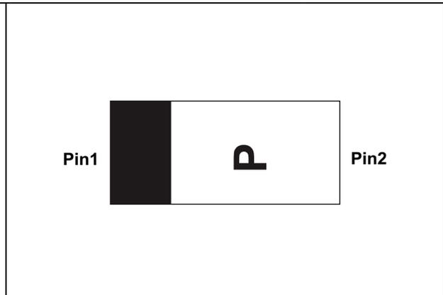
Note: The marking codes can be rotated by 90° or 180° to differentiate assembly location. In no case should this product marking be used to orient the component for its placement on a PCB. Only pin 1 mark is to be used for this purpose.
