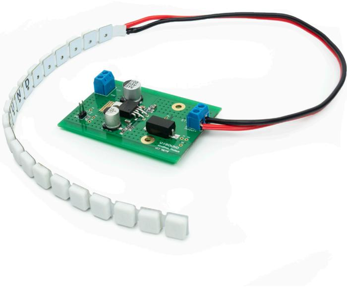
Dione Maxi consists of an array of MEMS speakers and the external amplifier to drive them. The speaker array, which is also referred to as the sound stripe, includes 20 USound Adap speakers connected in parallel. Due to its flexible structure and protective construction, the sound stripe is ideal for applications where audio is added on top of an existing design.
