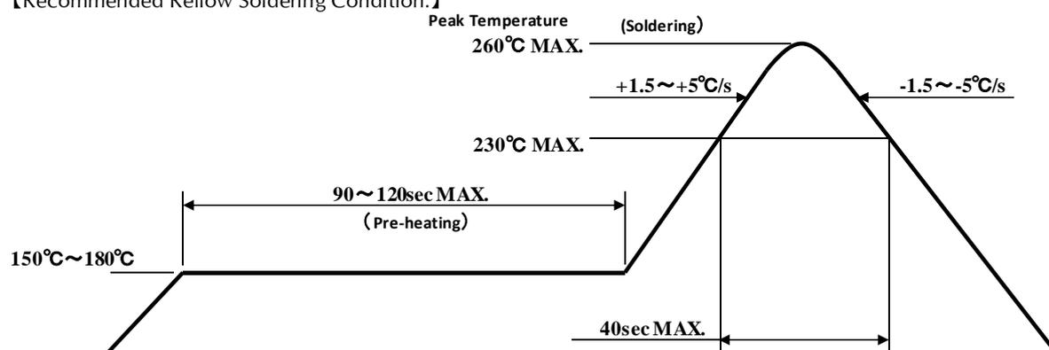
Note 1 Recommended temperature profile for the reflow soldering is listed as the temperature of the resin surface. This should be the maximum temperature for soldering. Lowering the heating temperature and decreasing heating time is very effective in achieving higher reliability.
