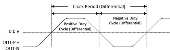
**Figure 37. HCSL Differential Measurement for Ringback**
