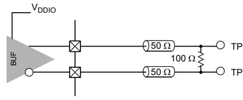
**Figure 25. CML Output Load and Test Circuit**
