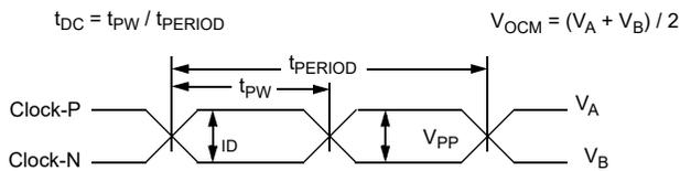
**Figure 31. Differential Output Definitions**
