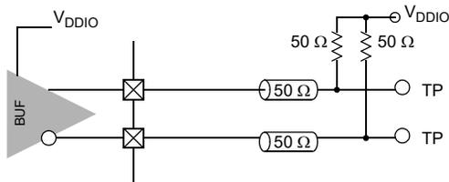
**Figure 26. HCSL Output Load and Test Circuit**
