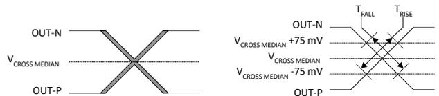
**Figure 36. HCSL Differential Measurement Point**
