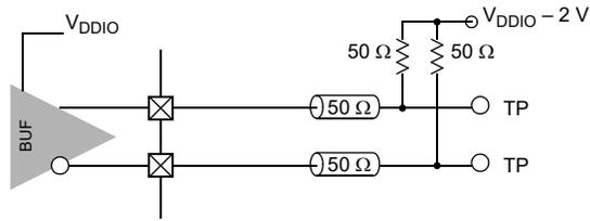
**Figure 24. LVDS Output Load and Test Circuit**
