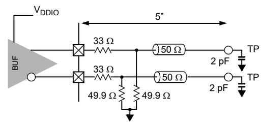
**Figure 27. LVCMOS Output Load and Test Circuit**
