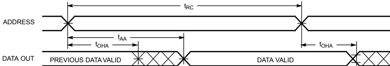
Figure 5. Read Cycle No. 2 (Either Port  $\overline{\text{CE}}/\overline{\text{OE}}$  Access) [26, 29, 30]
