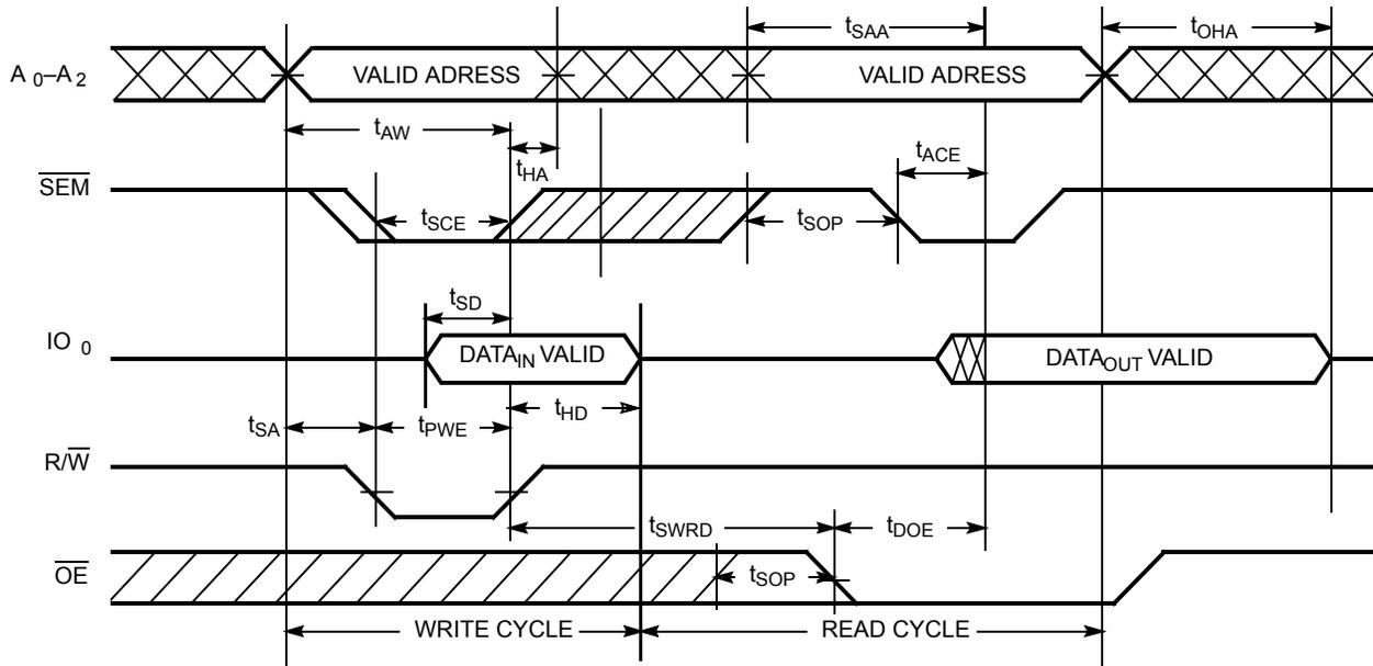
**Figure 10. Timing Diagram of Semaphore Contention** [41, 42, 43]
