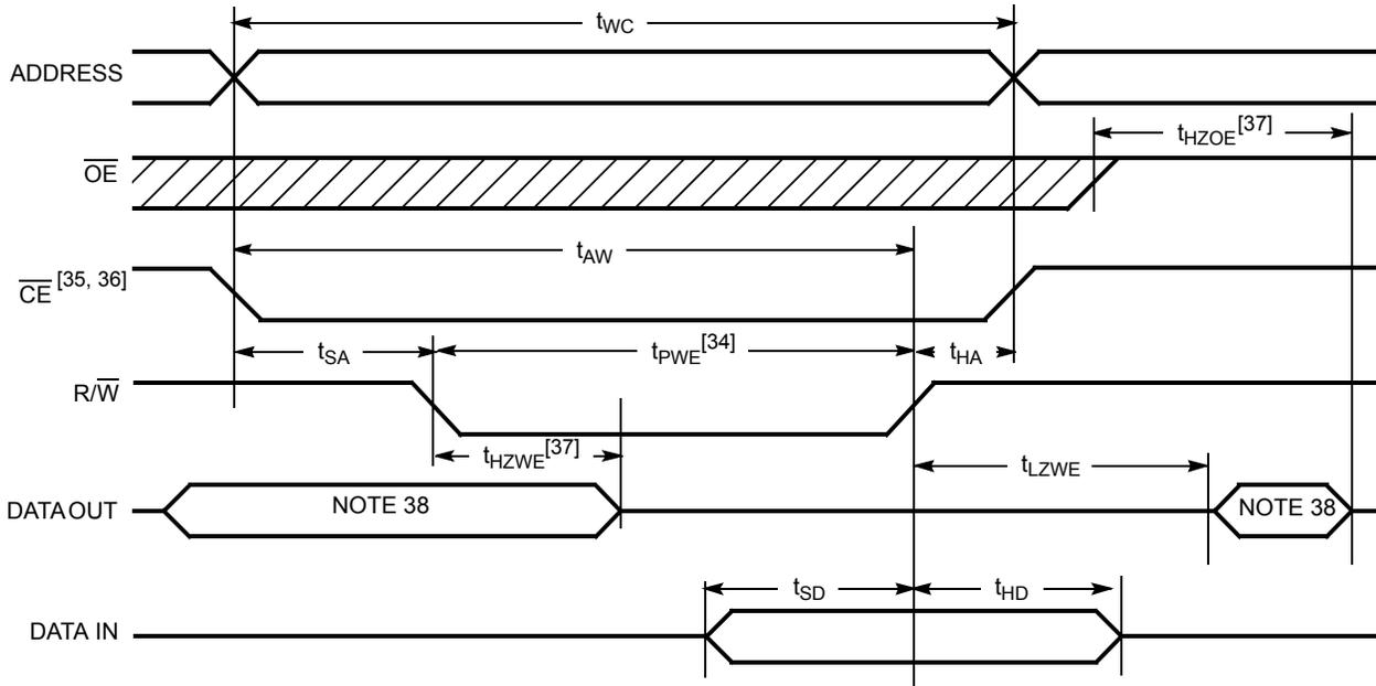
Figure 8. Write Cycle No. 2 (CE Controlled Timing) [31, 32, 33, 39]
