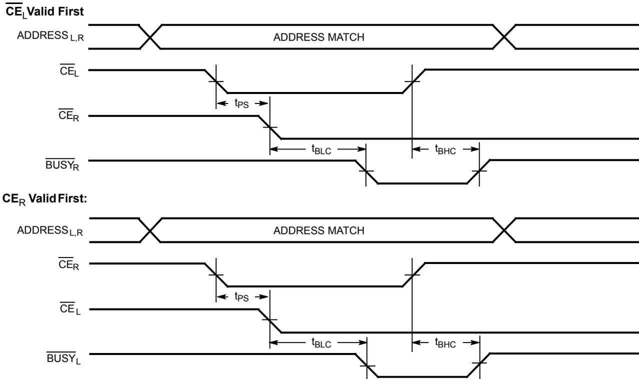
Figure 14. Busy Timing Diagram No.2 (Address Arbitration) [45]
