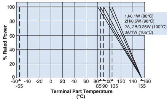
For resistors operated at a terminal part temperature of described for each size or above, a power rating shall be derated in accordance with the above derating curve.
