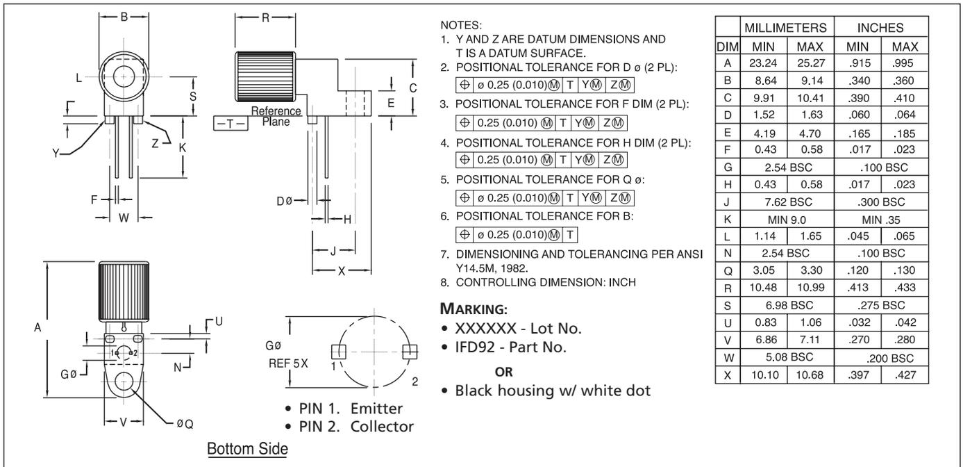
**FIGURE 4.** Case outline. Specifications are believed to be accurate but are subject to change. Industrial Fiber Optics assumes no responsibility for the consequences of using the information provided beyond replacement warranty for products not meeting stated specifications. Industrial Fiber Optics products are not authorized for use in life support applications without written approval from the President of Industrial Fiber Optics Corporation.
