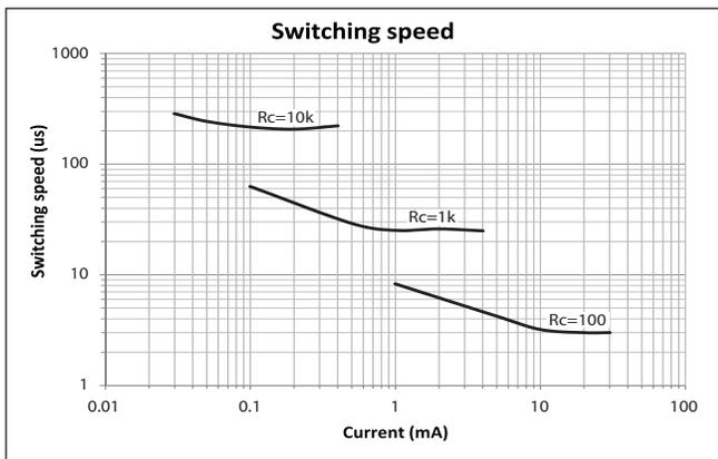
FIGURE 2. Rise and fall times of phototransistor.
