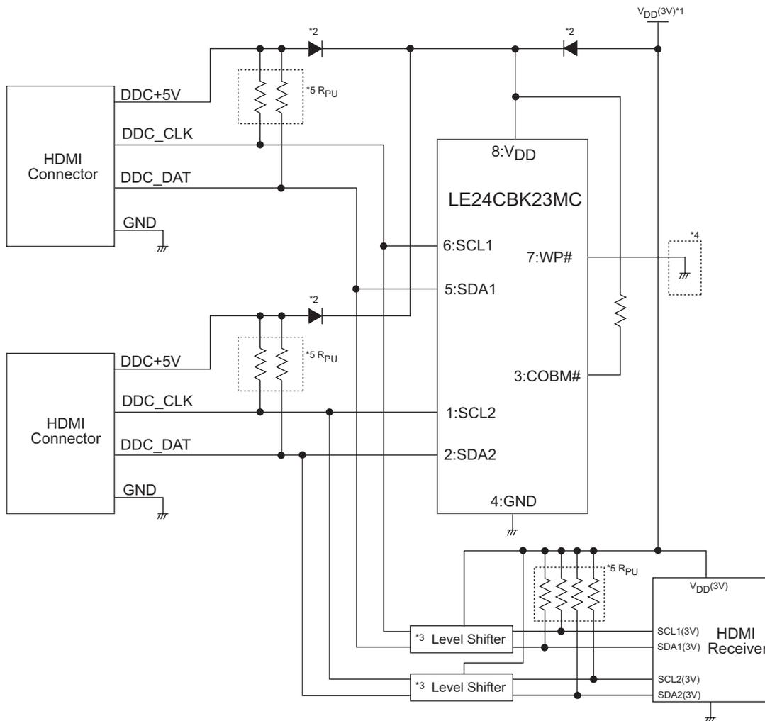
\*1: System power supply (3V) for HDMI receiver, etc.
