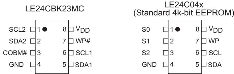
The Pin 3 (slave pin: S2) function of a regular 4K-bit EEPROM product is assigned to the COBM# pin of the LE24CBK23MC.
