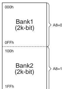
The MSB address in combined mode is A8. A8 is used to select the Bank1 or Bank2 area. Set A8 = 0 to control the Bank1 area, or A8 = 1 to control the Bank2 area.
