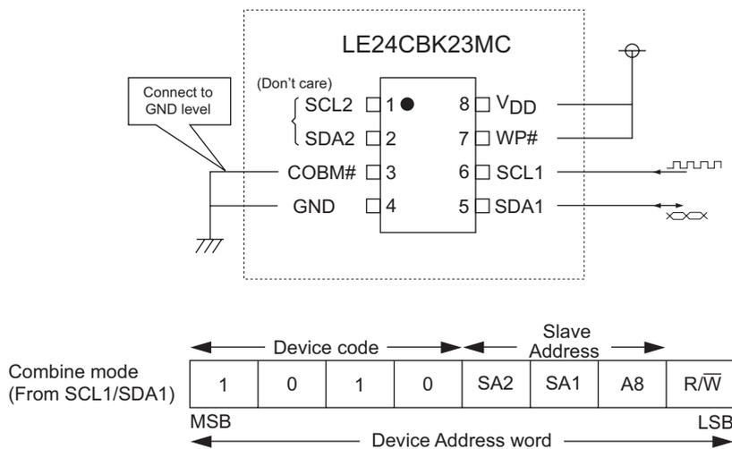
In combine mode, the slave address (SA2, SA1) is don't care, and any combination can be entered (SA2 = 1, SA1 = 1 or SA2 = 1, SA1 = 0 or SA2 = 0, SA1 = 1 or SA2 = 0, SA1 = 0).
