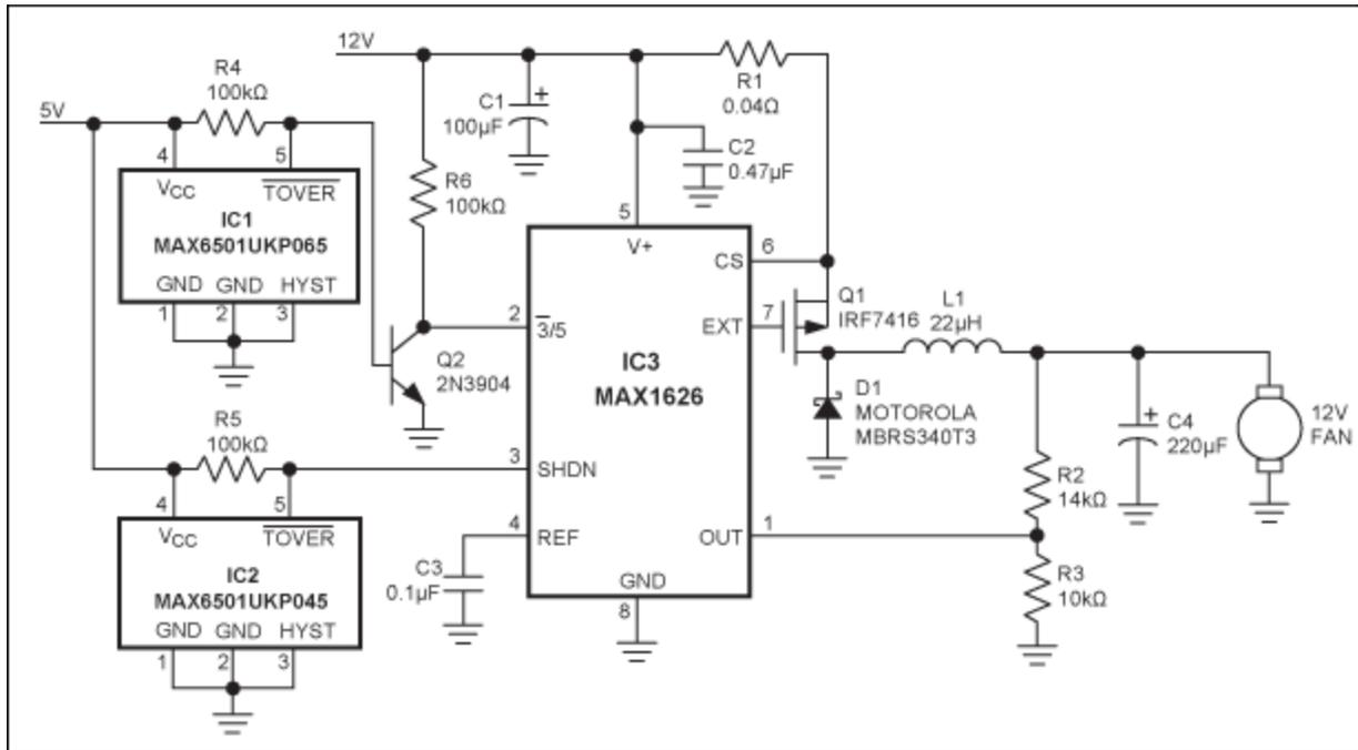
Figure 1. Controlled by the temperature monitors IC1 and IC2, this switch-mode DC-DC controller (IC3) applies either 0V, 8V, or 12V to the fan.
