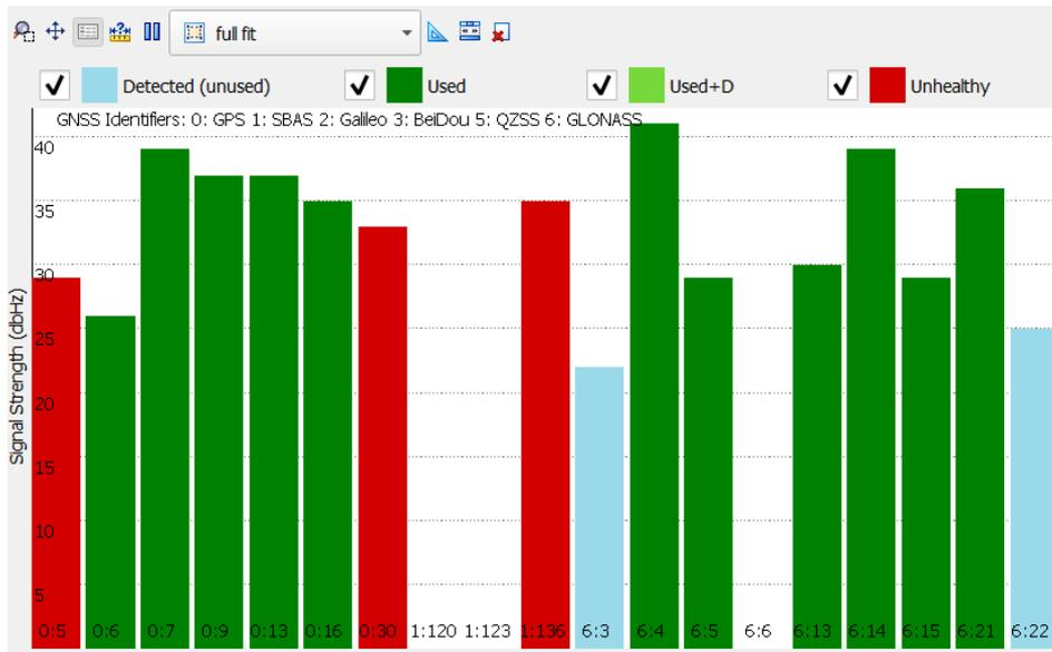
Figure 38 The SV info window showing 5 GPS satellites and 6 GLONASS satellites being used for the navigation solution and 2 satellites that have been detected.
