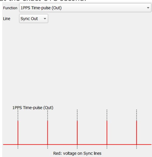
Figure 66: 1 PPS Time pulse in the Synchronization dialog
