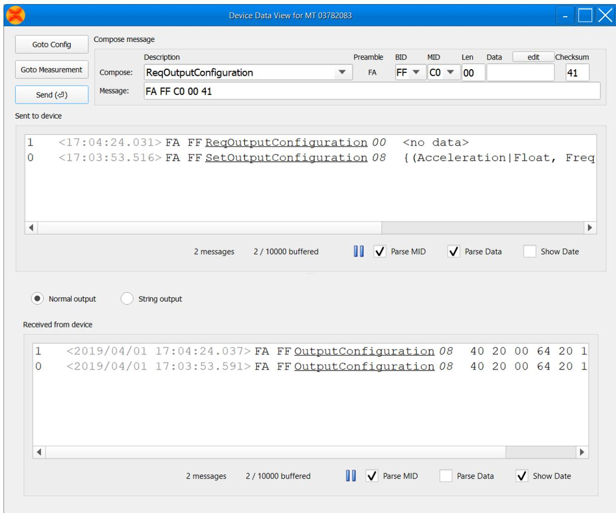
Figure 77: An example showing how to request settings from the MTi device.
