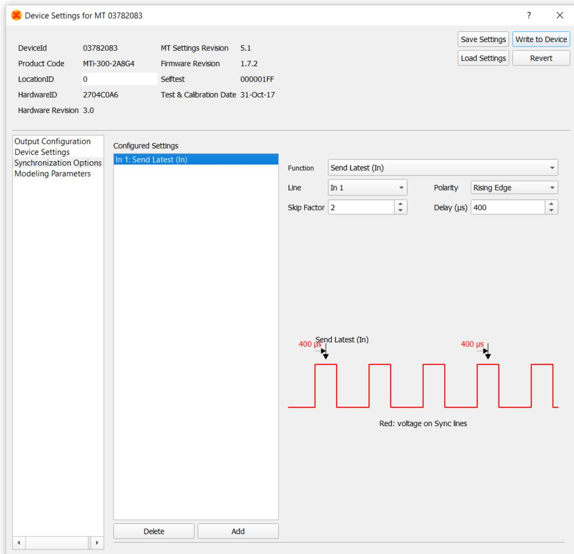
Figure 58: Starting the setup of a synchronization option.
