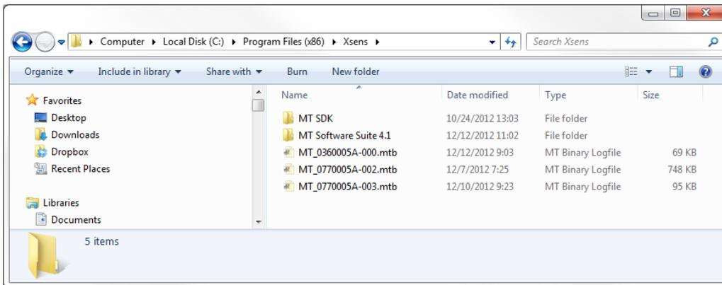
Figure 80: Log files of the MT Manager have an .mtb extension
