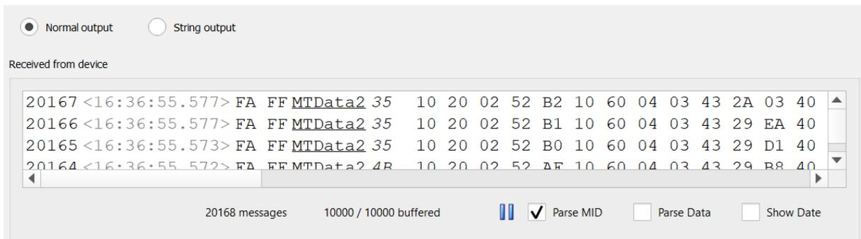
Figure 71: A typical view of received MTData2 messages shown in the Device Data View
