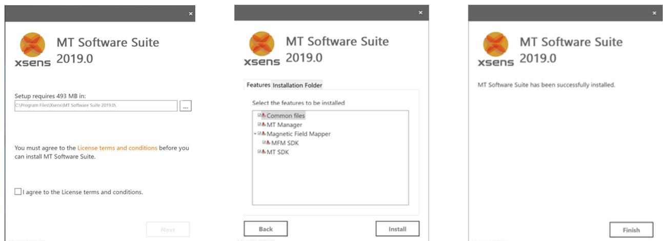
Figure 1: The installation procedure is straightforward. In the second screen, you can choose to skip installation of several components (not recommended)
