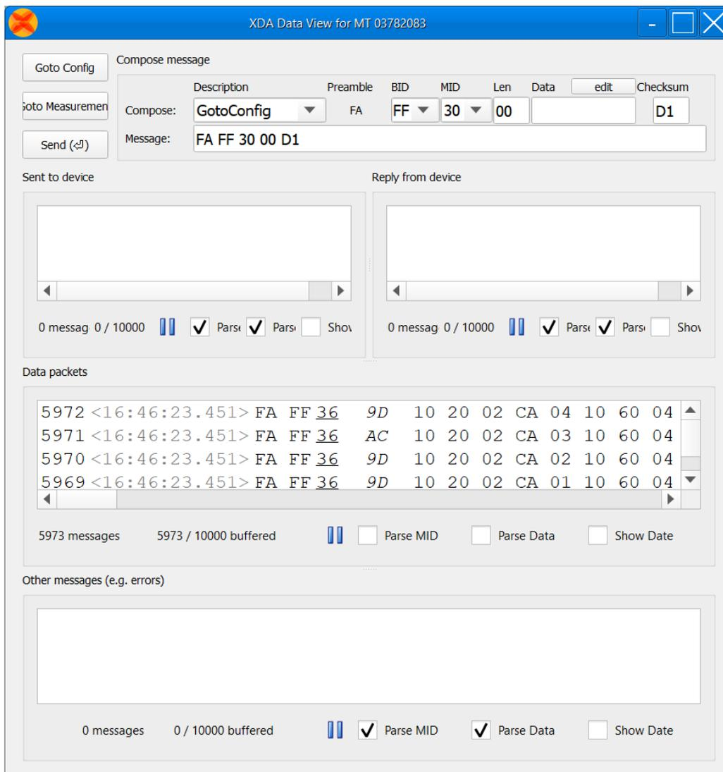
Figure 78: The XDA message terminal has an extra field with respect to the Device Data Viewer, showing the data received from the Xsens Device API (XDA)
