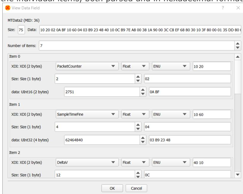
Figure 70: Double-clicking on the data will show the contents of a message, both parsed and in hexadecimal format
