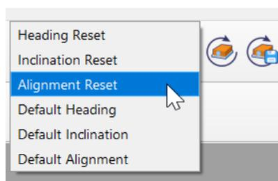
Figure 45: The orientation resets toolbar can be used to apply a specific reference coordinate system to the MTi's orientation, velocity and sensors data output
