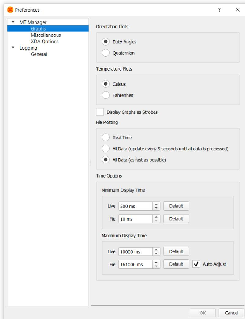
Figure 83: The behaviour of the graphs can be adapted in the Preferences - Graphs window
