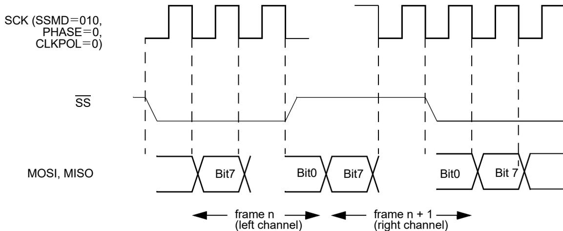
Figure 37. I<sup>2</sup>S Mode (SSMD=010), Multiple Frames
