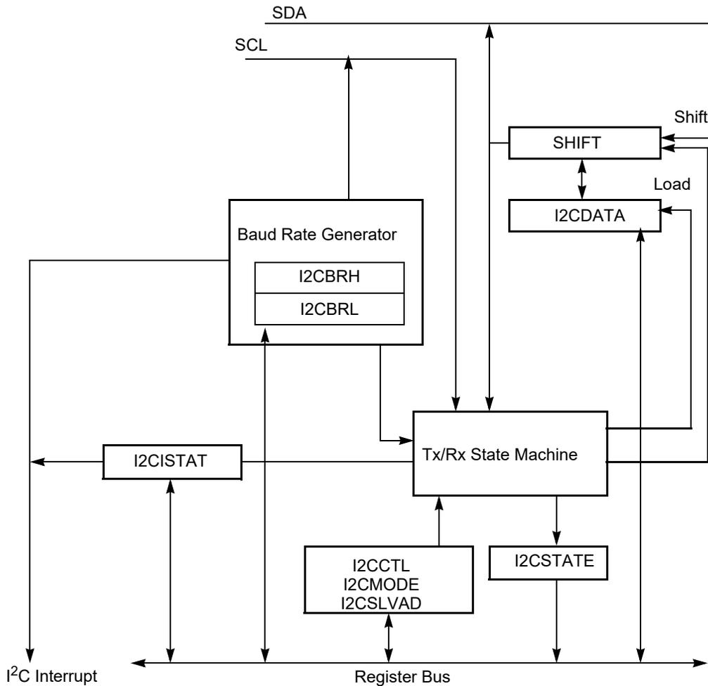
Figure 41. I<sup>2</sup>C Controller Block Diagram
