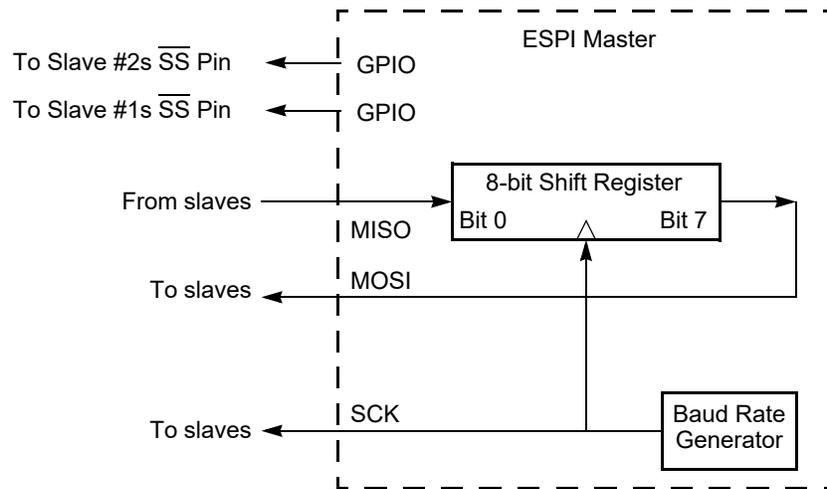
Figure 39. ESPI Configured as an SPI Master in a Single Master, Multiple Slave System
