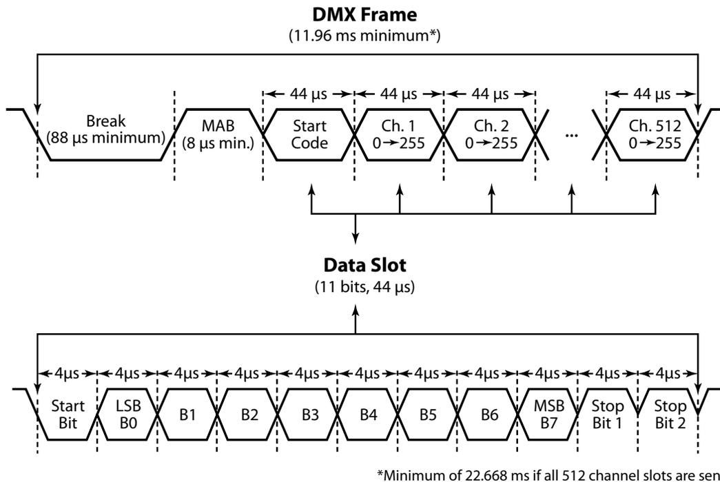
**Figure 29. UART-LDD DMX Frame and Data Slot**
