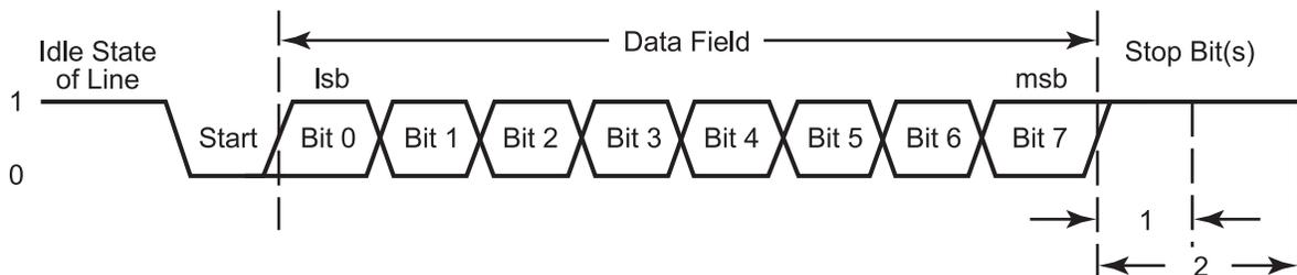
Figure 24. UART-LDD Asynchronous Data Format without Parity
