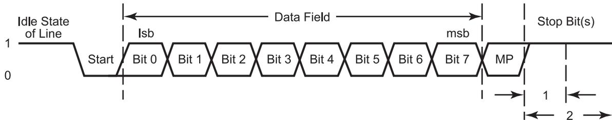
**Figure 27. UART-LDD Asynchronous Multiprocessor Mode Data Format**
