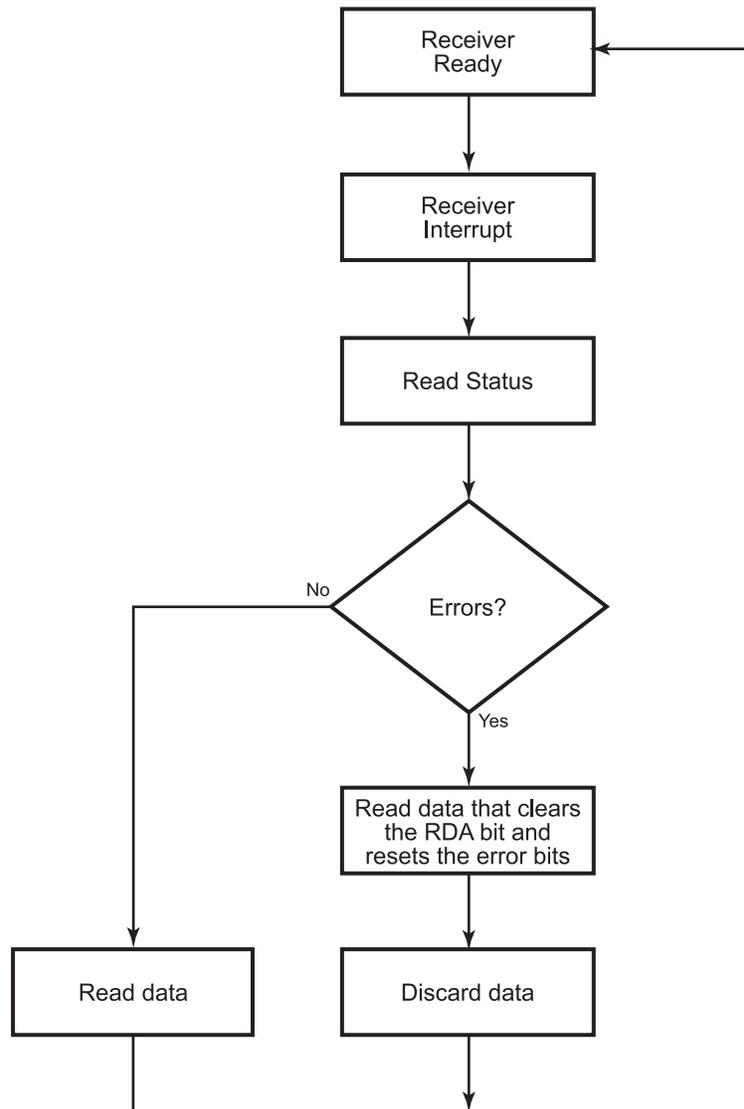
**Figure 30. UART-LDD Receiver Interrupt Service Routine Flow**
