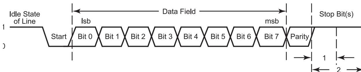
Figure 25. UART-LDD Asynchronous Data Format with Parity
