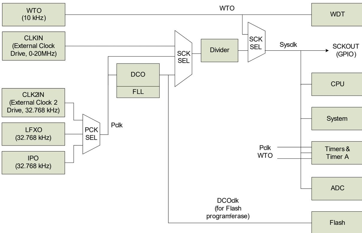
Figure 9. Clock System Block Diagram
