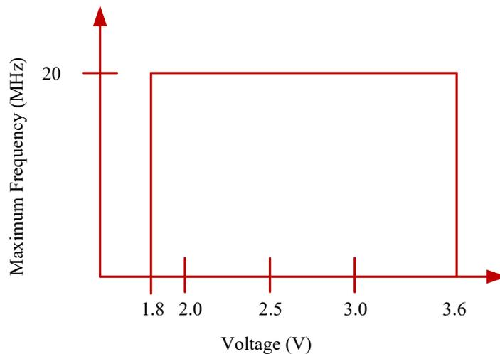
**Figure 71. Maximum System Clock Frequency vs.  $V_{DD}$**
