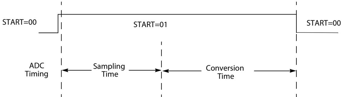
Figure 55. ADC Conversion Timing Diagram
