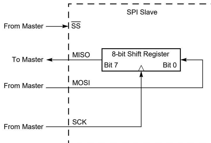
Figure 40. ESPI Configured as an SPI Slave
