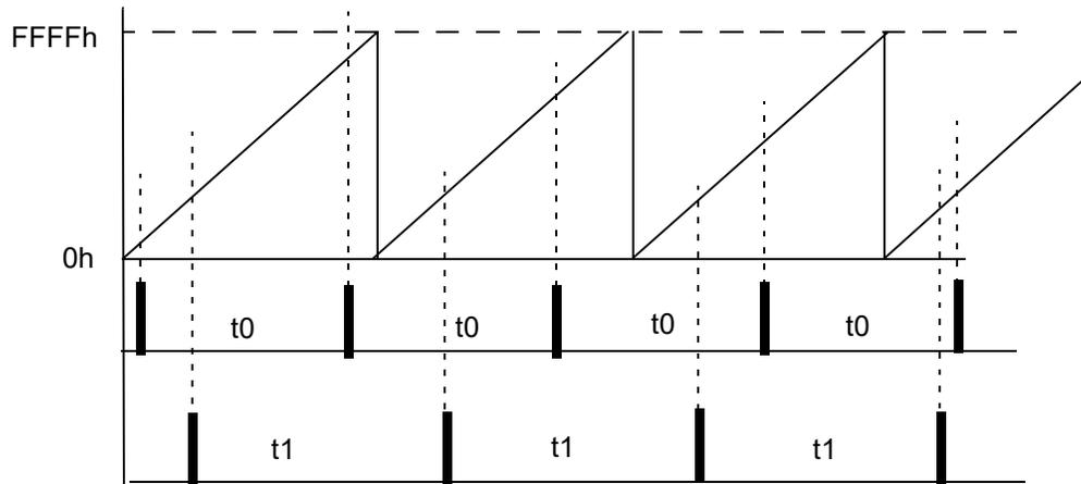
Figure 22. Count Max Mode with Channel Compare
