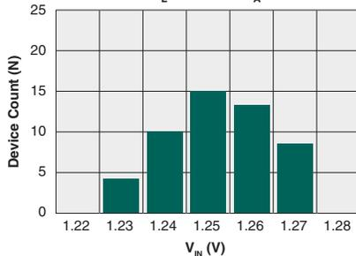
Typical  $V_{IN}$  for Switch Dropout
