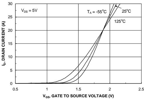
Figure 5. Transfer Characteristics.
