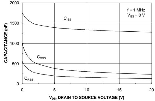
Figure 8. Capacitance Characteristics.
