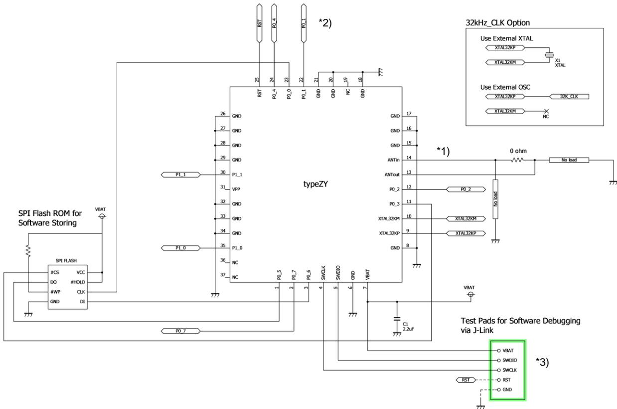
\*1) ANTout and ANTIn are to be connected with pi-matching network. Connected line is recommended to be as short as possible.
