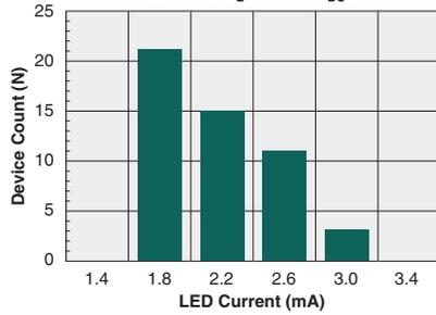
Typical  $I_F$  for Switch Dropout
