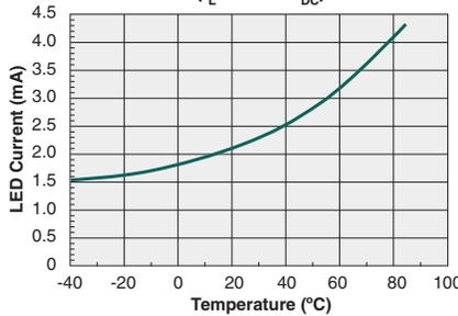
**Typical  $I_F$  for Switch Dropout vs. Temperature**
