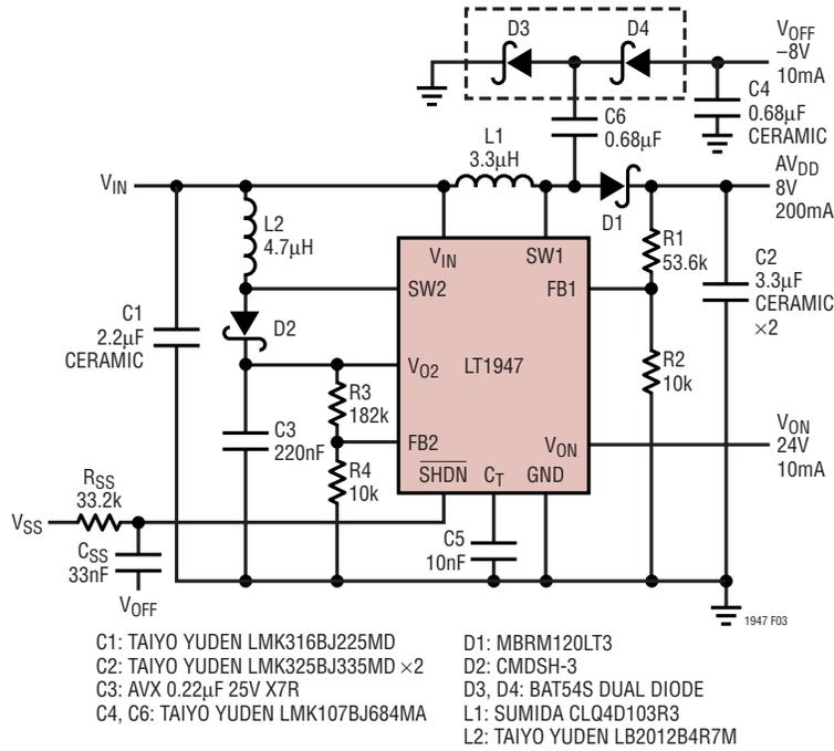
**Figure 3. R<sub>SS</sub> and C<sub>SS</sub> at SHDN Pin Provide Soft-Start**
