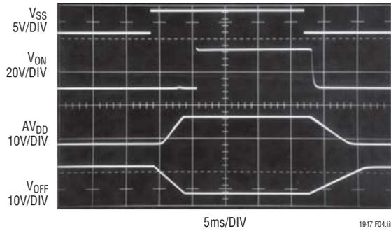
**Figure 4. Start-Up Waveforms with Soft-Start Circuit Added**
