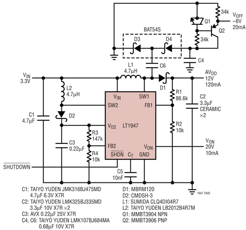
TFT-LCD Bias Generator: 10V, 24V, -6V Output
