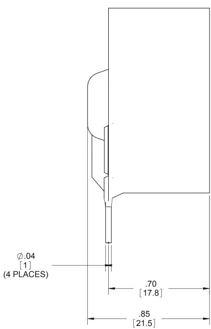
Tolerances: ± 0.02 in / 0.5 mm. All dimensions are in: inches [millimeters]
