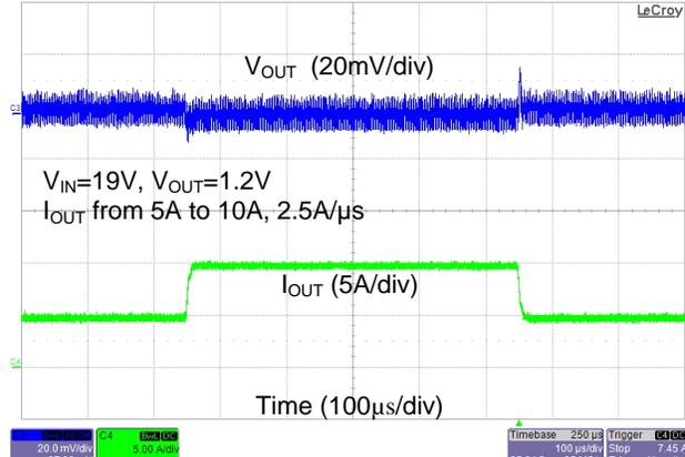
Figure 22. Load Transient from 50% to 100% Load Current
