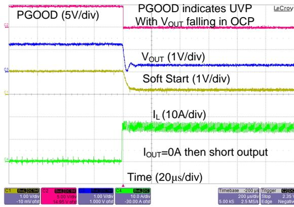
Figure 23. Over-Current Protection with Heavy Load Applied
