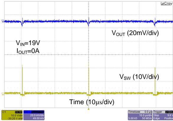
Figure 17. Static Load Ripple at Light Load
