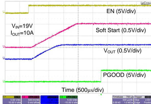
Figure 14. Startup Waveforms with 10 A Load Current
