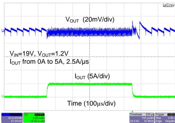
Figure 21. Load Transient from 0% to 50% Load Current
