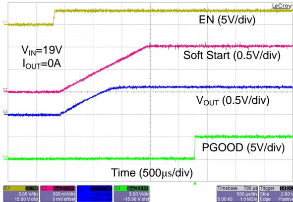
Figure 13. Startup Waveforms with 0 A Load Current
