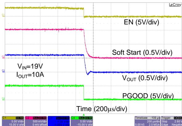
Figure 15. Shutdown Waveforms with 10 A Load Current
