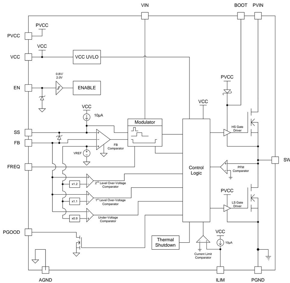
Figure 2. Block Diagram
