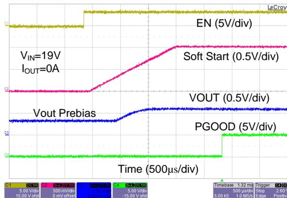
Figure 16. Startup Waveforms with Prebias Voltage on Output
