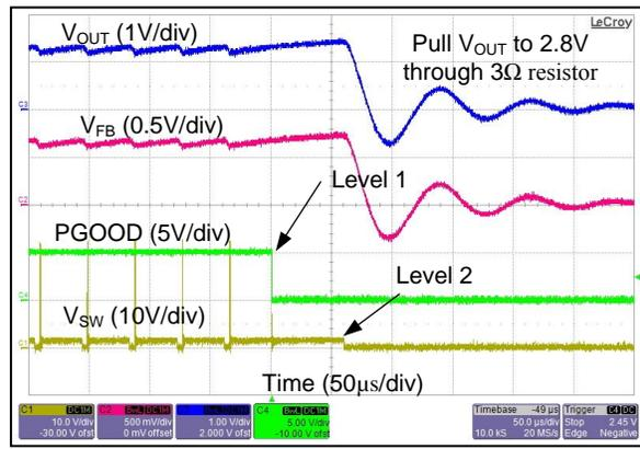
Figure 24. Over-Voltage Protection Level 1 and Level 2
