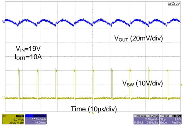
Figure 18. Static Load Ripple at Full Load
