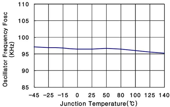
Figure 7. Oscillator Frequency
