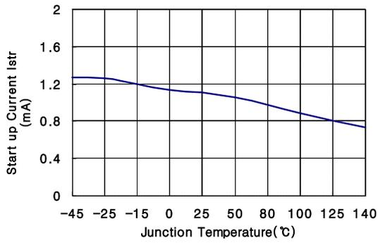
Figure 11. Startup Current
