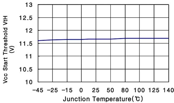
Figure 5. V<sub>CC</sub> Start Threshold Voltage
