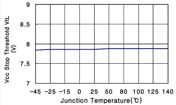
Figure 6. V<sub>CC</sub> Stop Threshold Voltage
