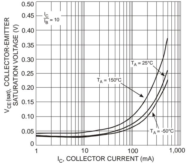
Figure 5 Collector-Emitter Saturation Voltage vs. Collector Current
