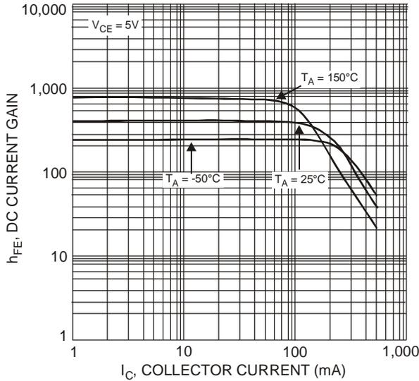
Figure 4 Typical DC Current Gain vs. Collector Current
