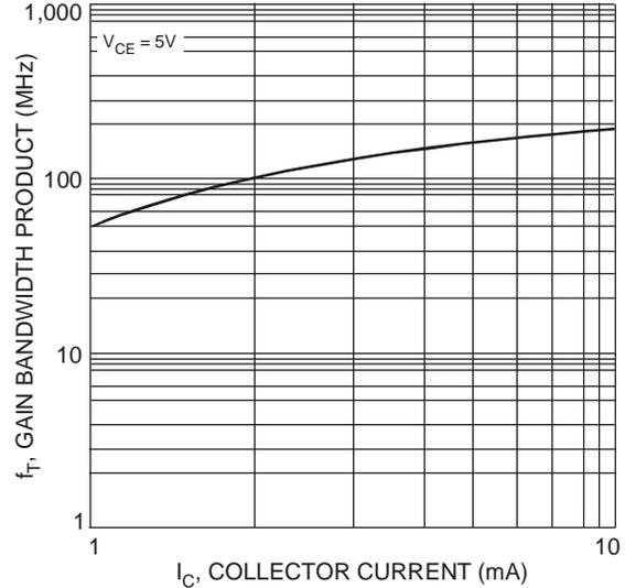
Figure 7 Typical Gain Bandwidth Product vs. Collector Current
