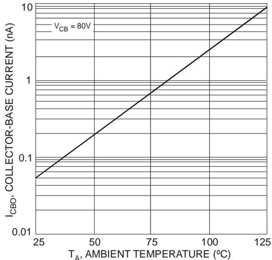
Figure 8 Typical Collector-Cutoff Current vs. Ambient Temperature
