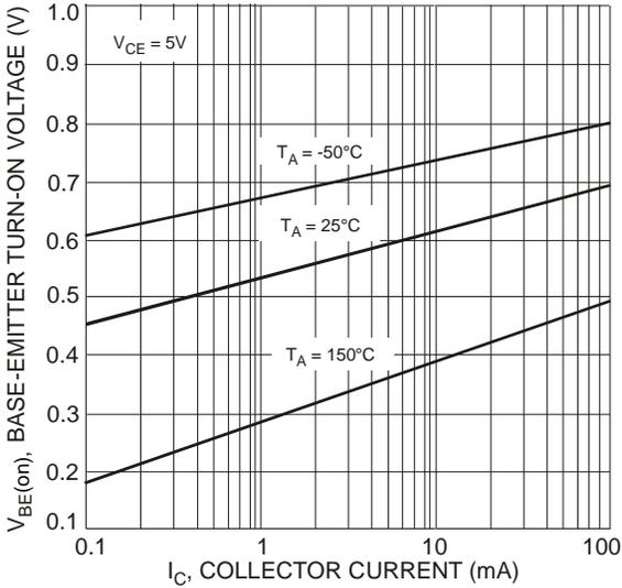
Figure 6 Typical Base-Emitter Turn-On Voltage vs. Collector Current
