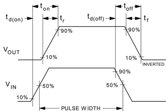
**Figure 12. Switching Waveforms.**
