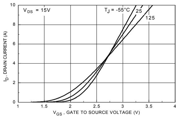
Figure 5. Transfer Characteristics.
