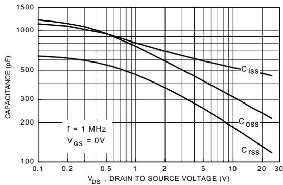
**Figure 9. Capacitance Characteristics.**
