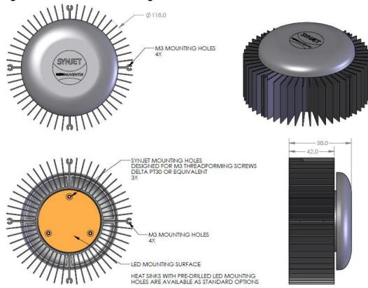
CUSTOMER-CONFIGURABLE VERSION WITH COPPER INSERT SHOWN
