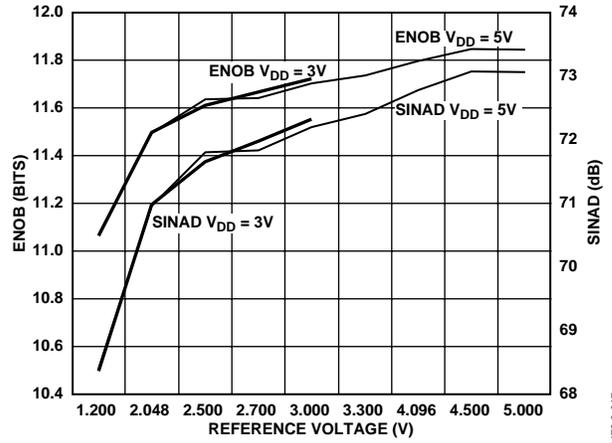
Figure 17. AD7994 SINAD/ENOB vs. Reference Voltage, Mode 1, 121 kSPS
