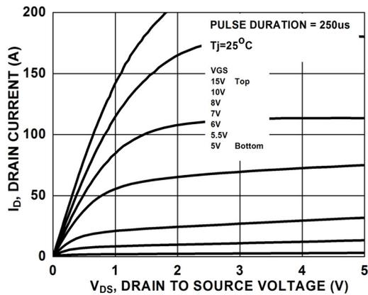
Figure 9. Saturation Characteristics
