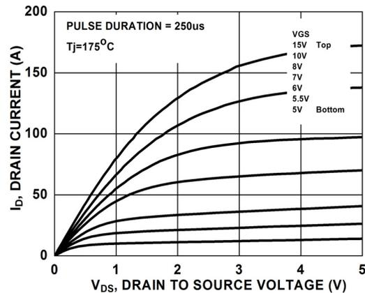
Figure 10. Saturation Characteristics
