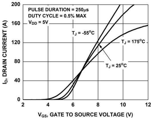
Figure 7. Transfer Characteristics
