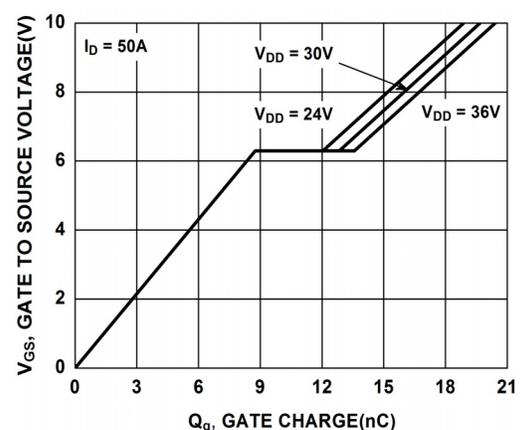
Figure 16. Gate Charge vs. Gate to Source Voltage
