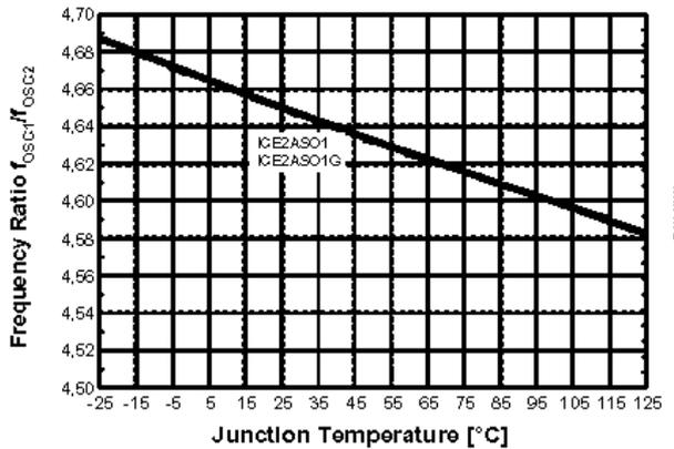
Figure 34 Frequency Ratio  $f_{OSC1} / f_{OSC2}$  vs.  $T_j$
