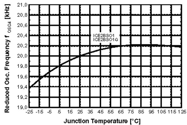
Figure 33 Reduced Osc. Frequency  $f_{OSC4}$  vs.  $T_j$
