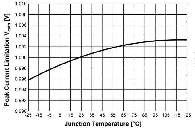
Figure 44 Peak Current Limitation  $V_{csth}$  vs.  $T_j$
