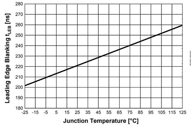
Figure 45 Leading Edge Blanking  $V_{VCC1}$  vs.  $T_j$
