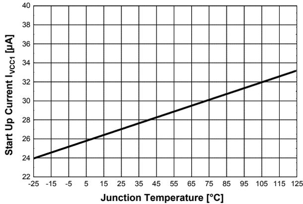
Figure 23 Start Up Current  $I_{VCC1}$  vs.  $T_j$
