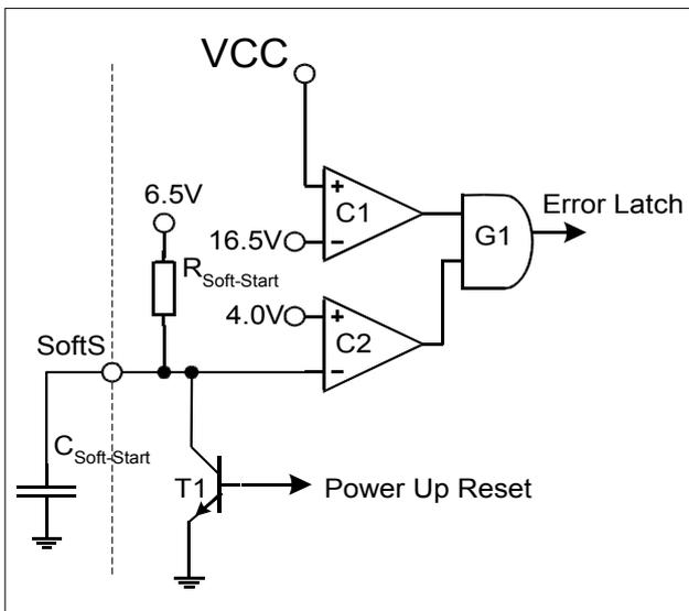
Figure 22 Overvoltage Detection
