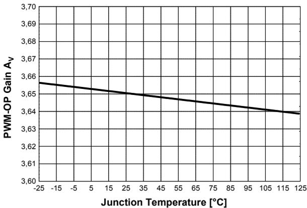
Figure 37 PWM-OP Gain  $A_V$  vs.  $T_j$
