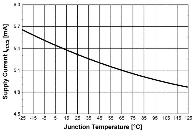
Figure 24 Supply Current  $I_{VCC2}$  vs.  $T_j$
