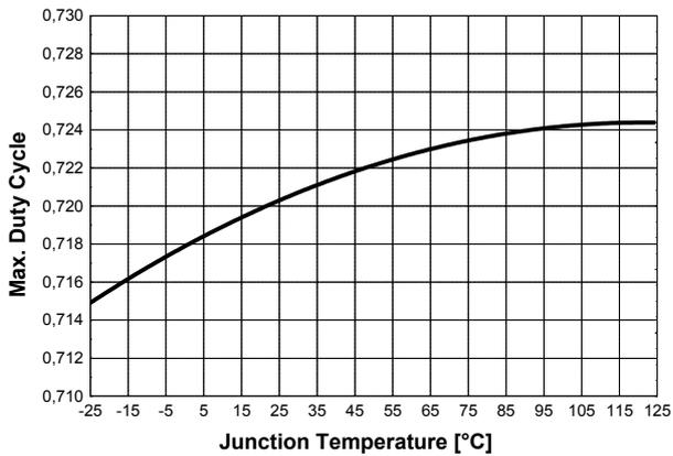
Figure 36 Max. Duty Cycle vs.  $T_j$
