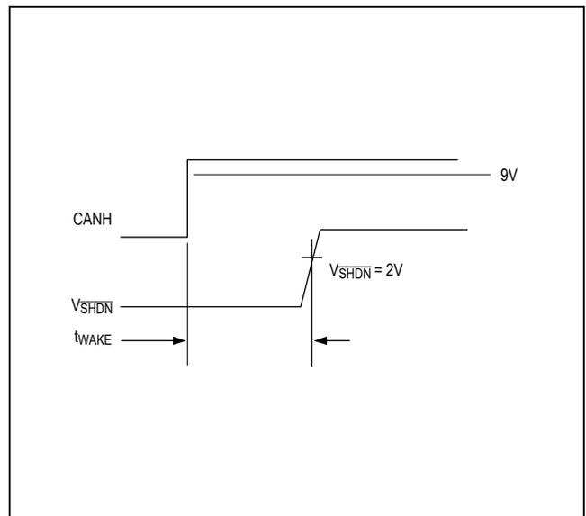
Figure 3. Time to Wakeup ( $t_{wake}$ )
