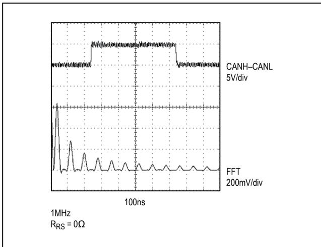
Figure 7. Output Bus High-Speed Mode at 2Mbps
