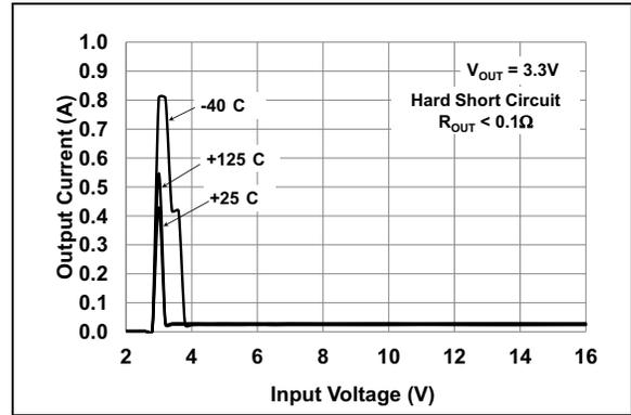
**FIGURE 2-16:** Short Circuit Current vs. Input Voltage.
