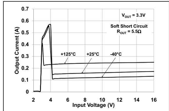
**FIGURE 2-17:** Short Circuit Current vs. Input Voltage.
