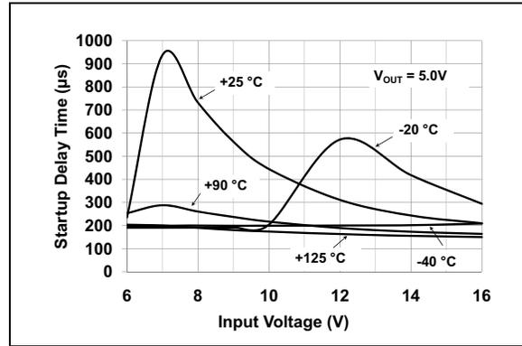
**FIGURE 2-34:** Start-up Delay From SHDN to 90%  $V_{OUT}$ .
