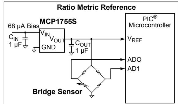
FIGURE 5-2: Using the MCP1755/1755S as a Voltage Reference.
