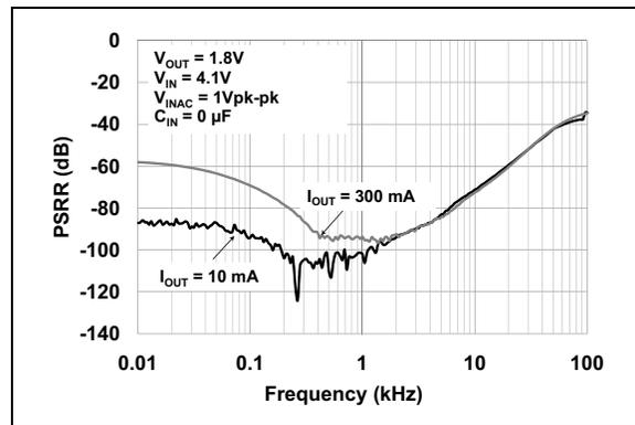
**FIGURE 2-24:** Power Supply Ripple Rejection vs. Frequency.
