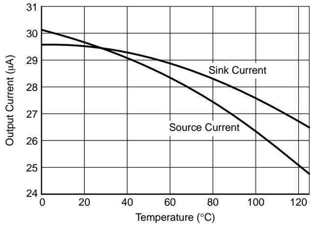
Figure 10. Error Amp Output Currents vs. Temperature
