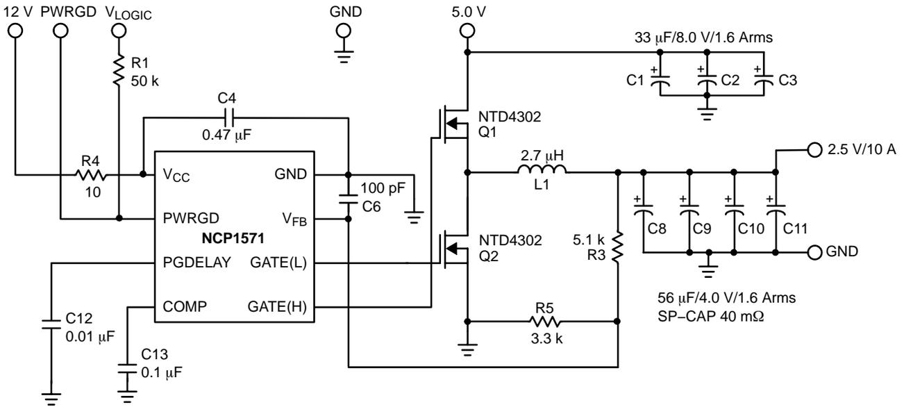
Figure 1. Applications Circuit
