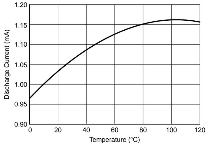
Figure 12. COMP Fault Mode Discharge Current vs. Temperature
