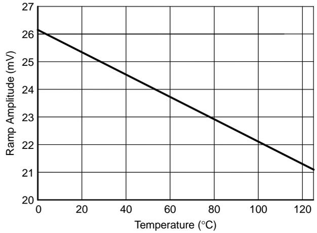
Figure 6. Artificial Ramp Amplitude vs. Temperature (50% Duty Cycle)
