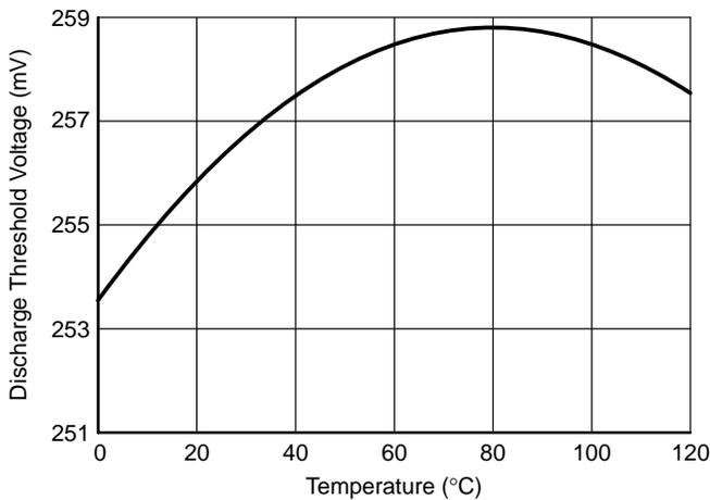
Figure 19. PGDELAY Discharge Threshold Voltage vs. Temperature
