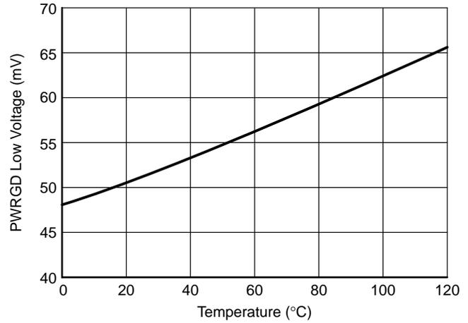
Figure 16. PWRGD Output Low Voltage vs. Temperature
