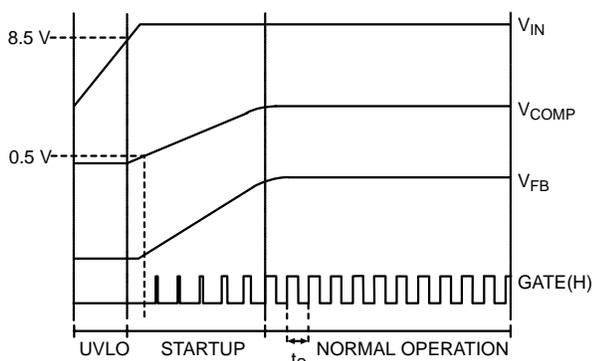
Figure 22. Idealized Waveforms
