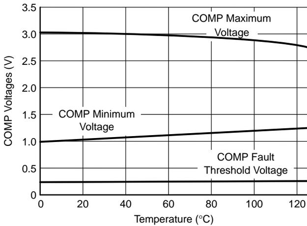
Figure 11. COMP Voltages vs. Temperature
