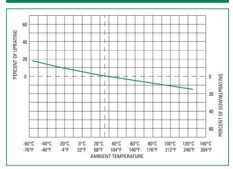
Note: Rerating depicted in this curve is in addition to the standard derating of 25% for continuous operation.
