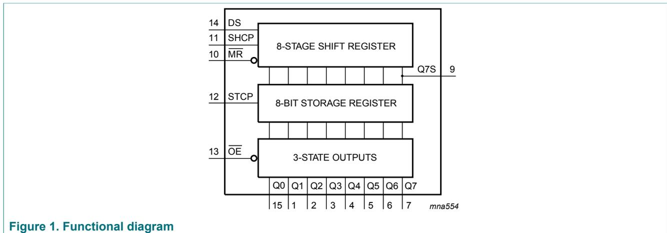
Figure 1. Functional diagram
