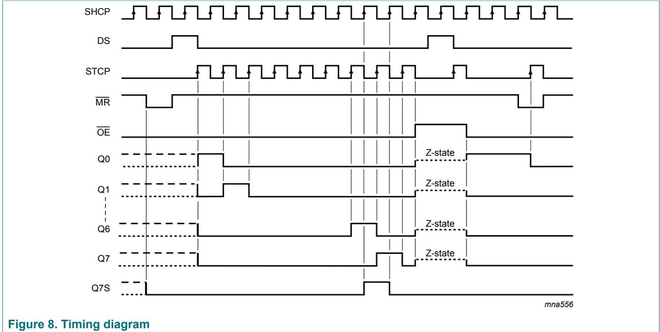
Figure 8. Timing diagram
