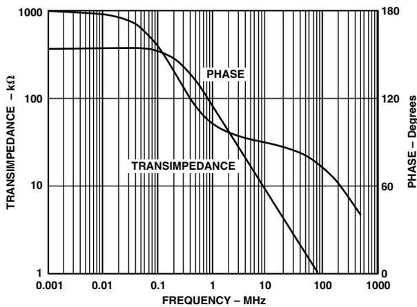
TPC 28. Open-Loop Transimpedance and Phase vs. Frequency
