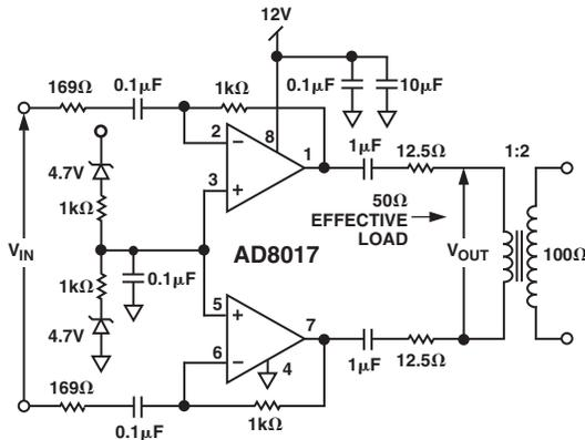
Figure 7. Single 12 V Supply ADSL Remote Terminal Transmitter
