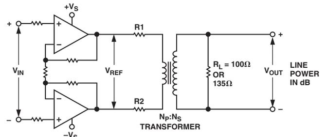
Figure 2. Differential Drive Circuit for xDSL Applications
