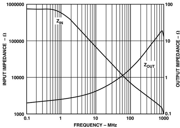
TPC 31. Input and Output Impedance vs. Frequency
