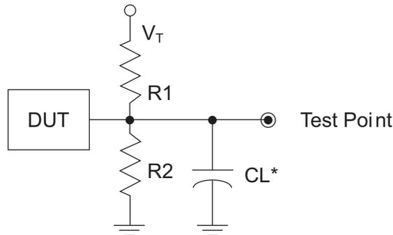
\*CL Includes Test Fixture and Probe Capacitance
