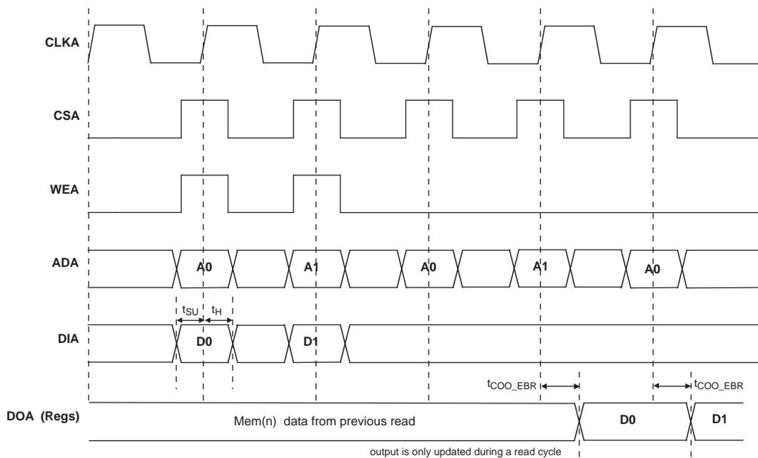
Figure 3-8. Write Through (SP Read/Write on Port A, Input Registers Only)
