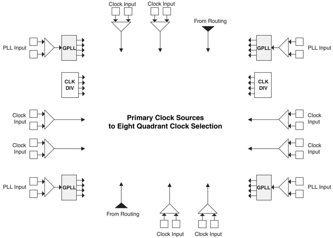
Note: This diagram shows sources for the XP2-17 device. Smaller LatticeXP2 devices have two GPLLs.
