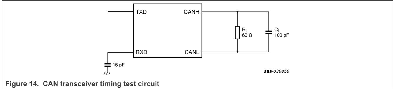
Figure 14. CAN transceiver timing test circuit
