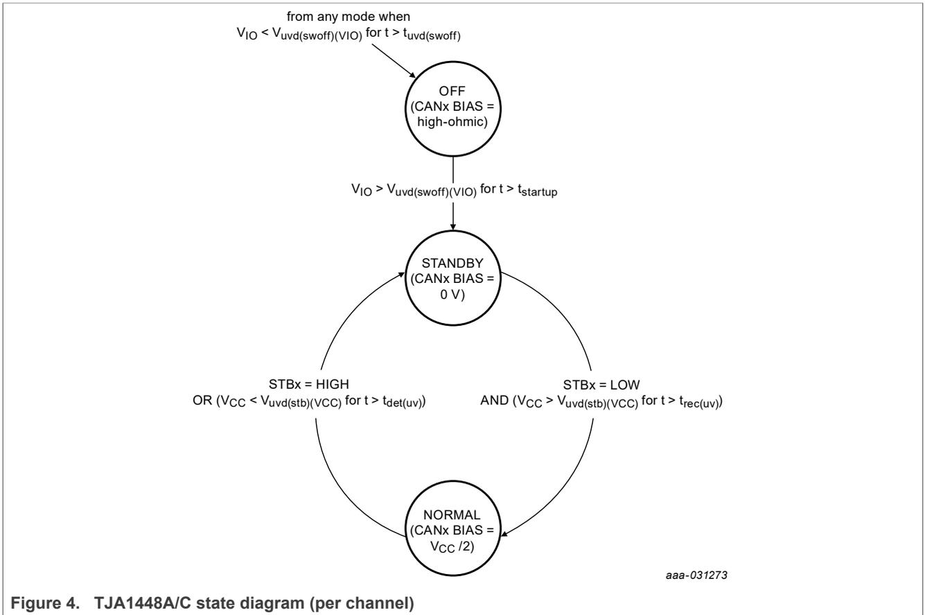
Figure 4. TJA1448A/C state diagram (per channel)
