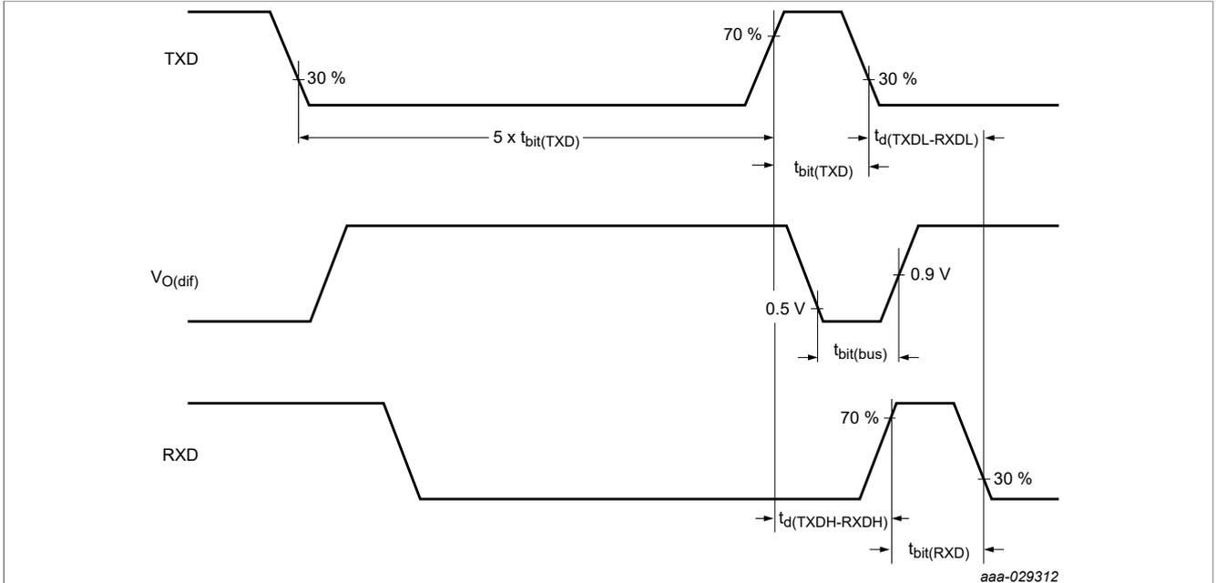
Figure 10. CAN FD timing definitions according to ISO 11898-2:2016
