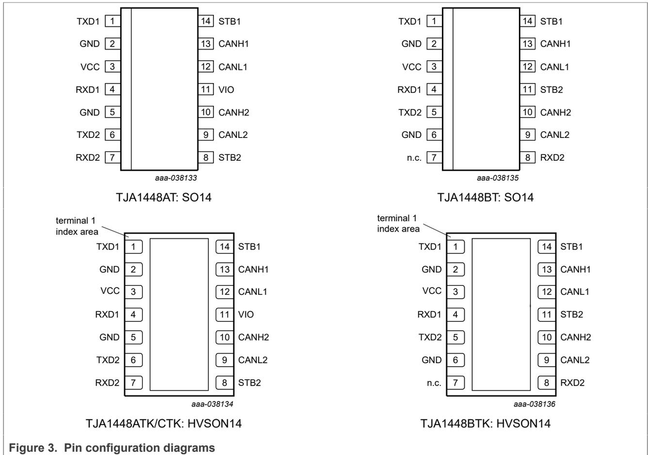
Figure 3. Pin configuration diagrams
