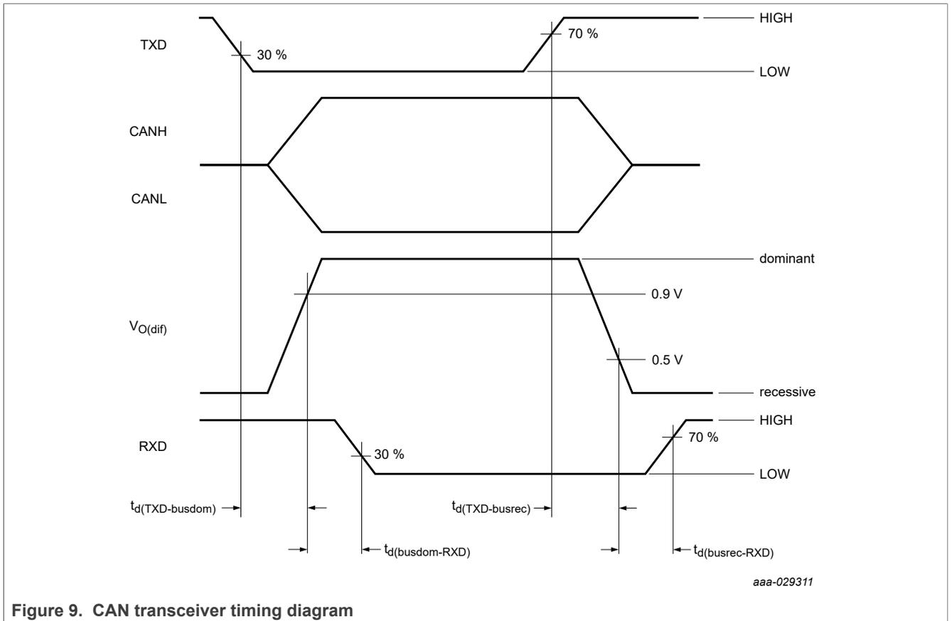
Figure 9. CAN transceiver timing diagram
