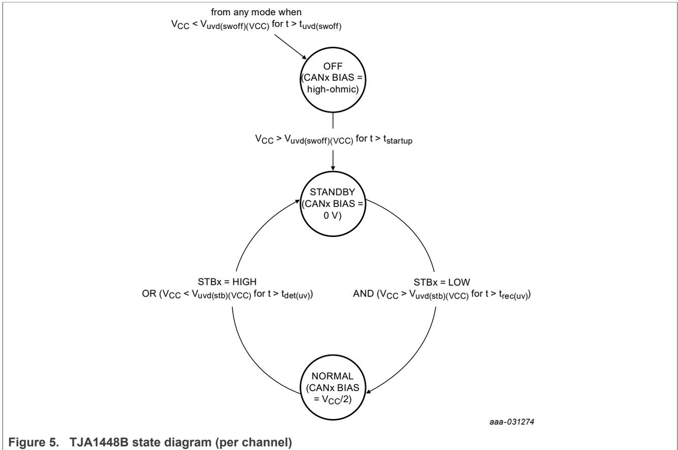
Figure 5. TJA1448B state diagram (per channel)
