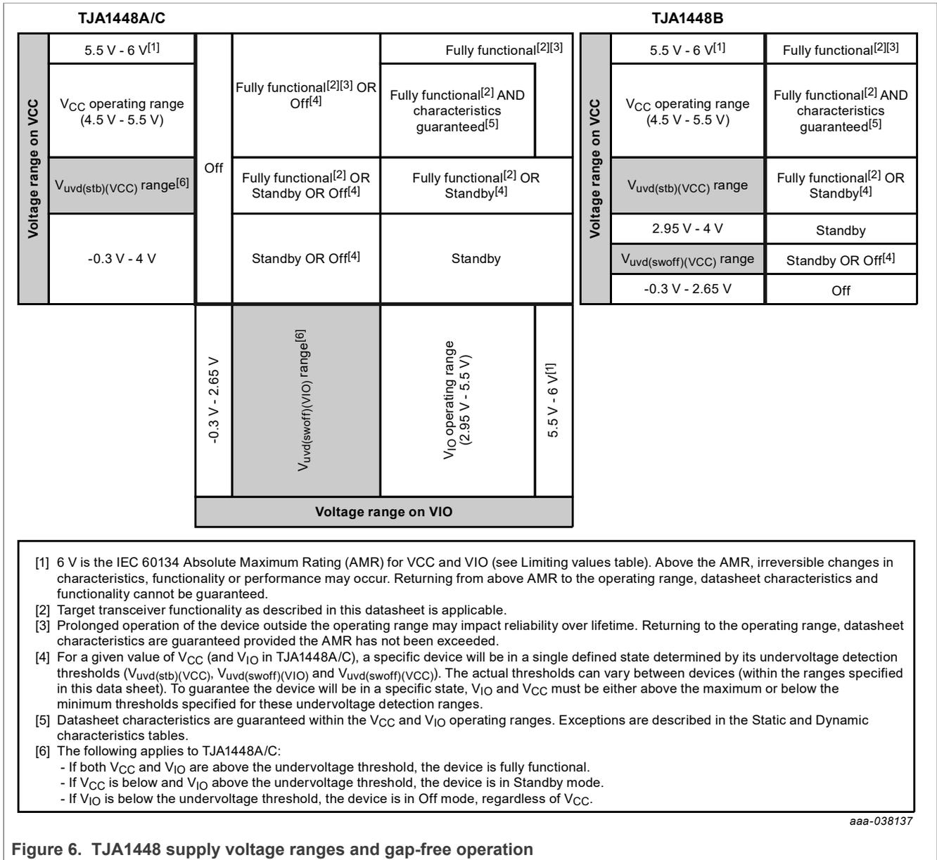
Figure 6. TJA1448 supply voltage ranges and gap-free operation
