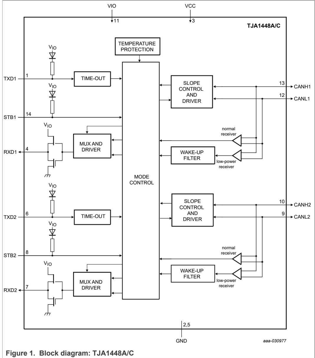
Figure 1. Block diagram: TJA1448A/C
