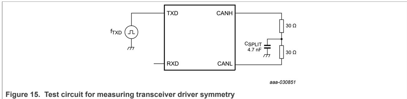
Figure 15. Test circuit for measuring transceiver driver symmetry
