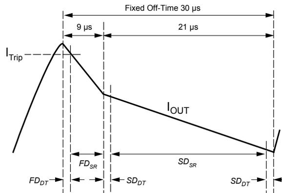
Figure 2. Mixed Decay Mode Operation
