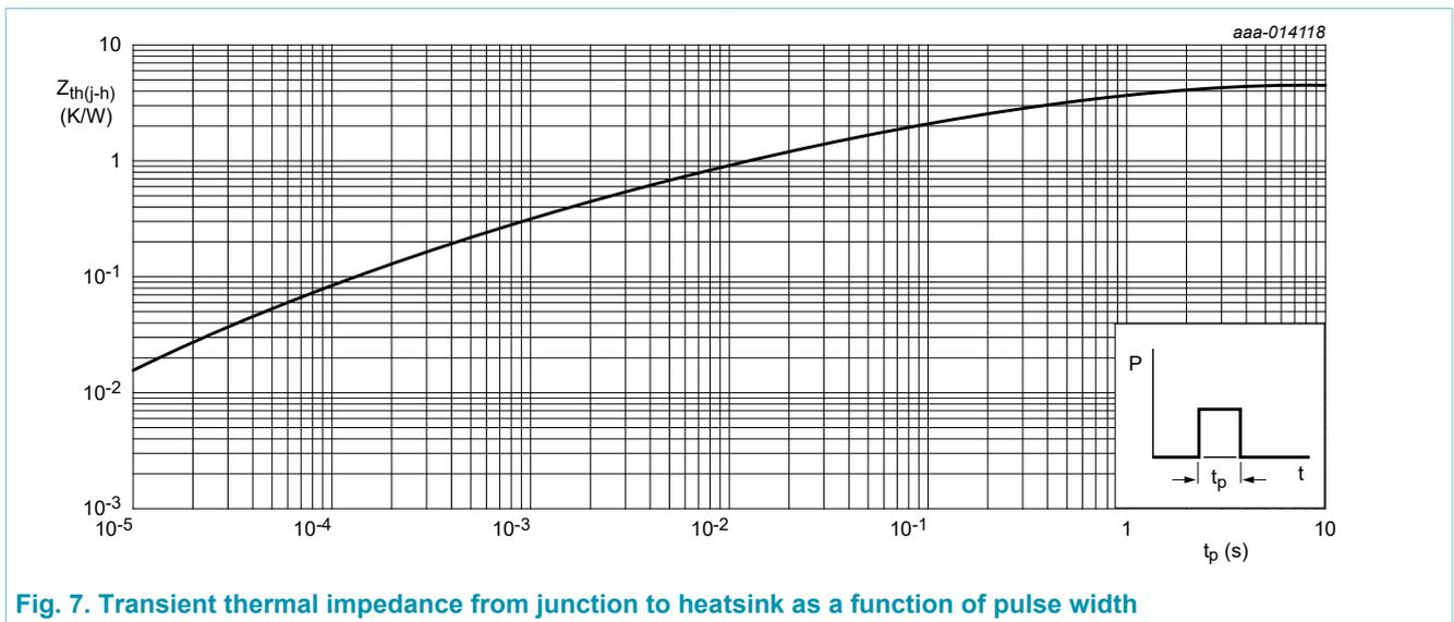
Fig. 7. Transient thermal impedance from junction to heatsink as a function of pulse width
