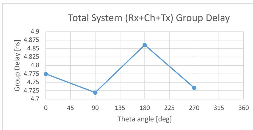
The measured Group Delay variation for the FXUBW01 antenna is 141ps as can be seen in the graph above Figure.
