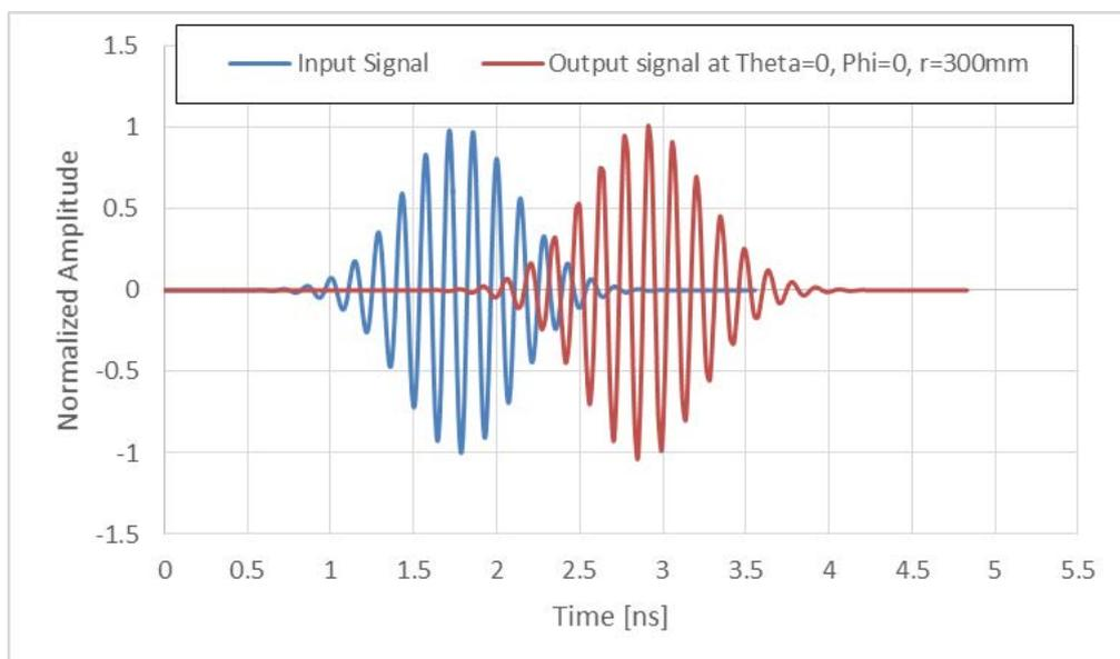
Fidelity of signals as above is calculated and results as below are obtained. The values are well above 0.9 and it is considered that antenna has very good performance.
