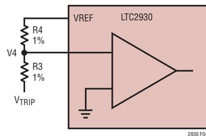
Figure 4. Setting the Negative Adjustable Trip Point
