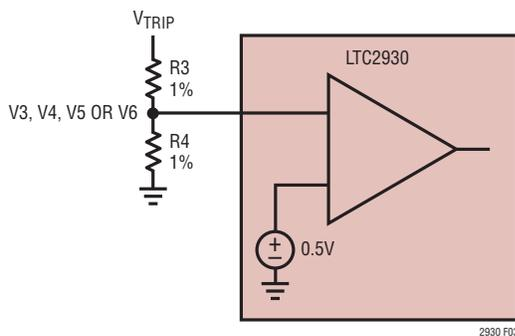
Figure 3. Setting the Positive Adjustable Trip Point
