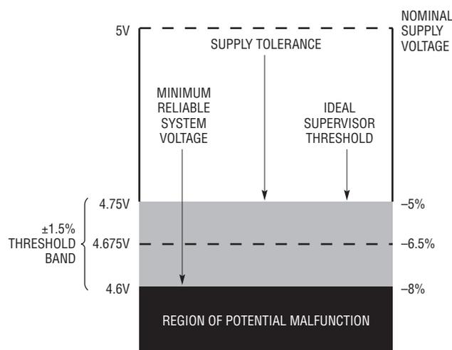
Figure 1. 1.5% Threshold Accuracy Improves System Reliability
