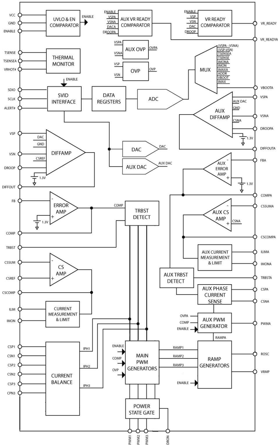
Figure 1. Block Diagram
