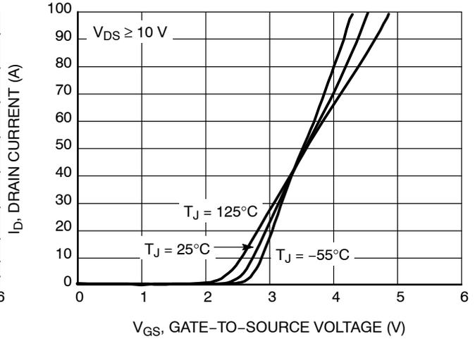
Figure 2. Transfer Characteristics
