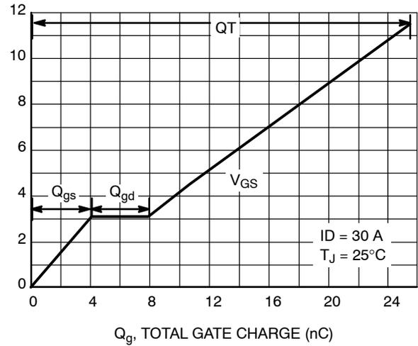
Figure 8. Gate-to-Source and Drain-to-Source Voltage vs. Total Charge
