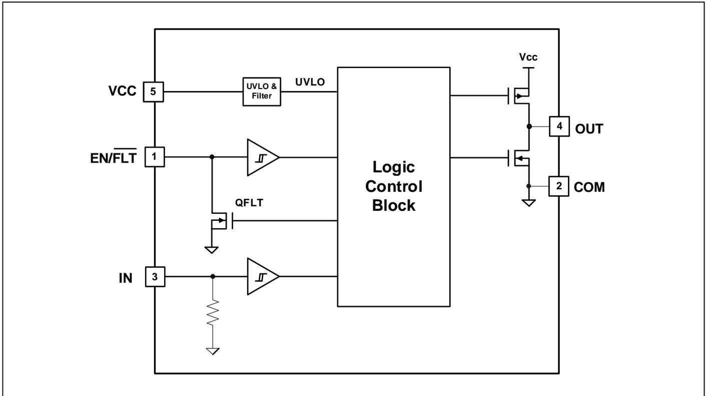
Figure 2 Block diagram
