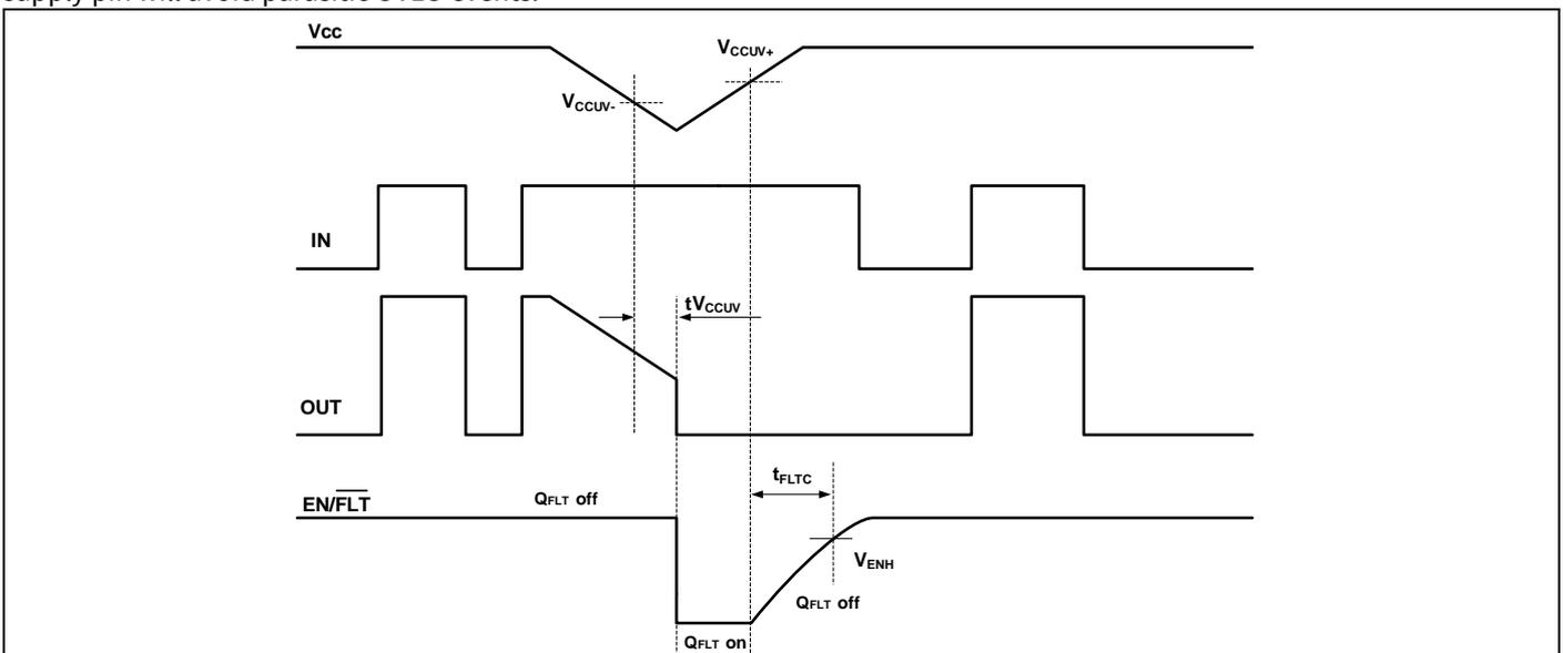
Figure 8 VCC under voltage protection waveform definitions
