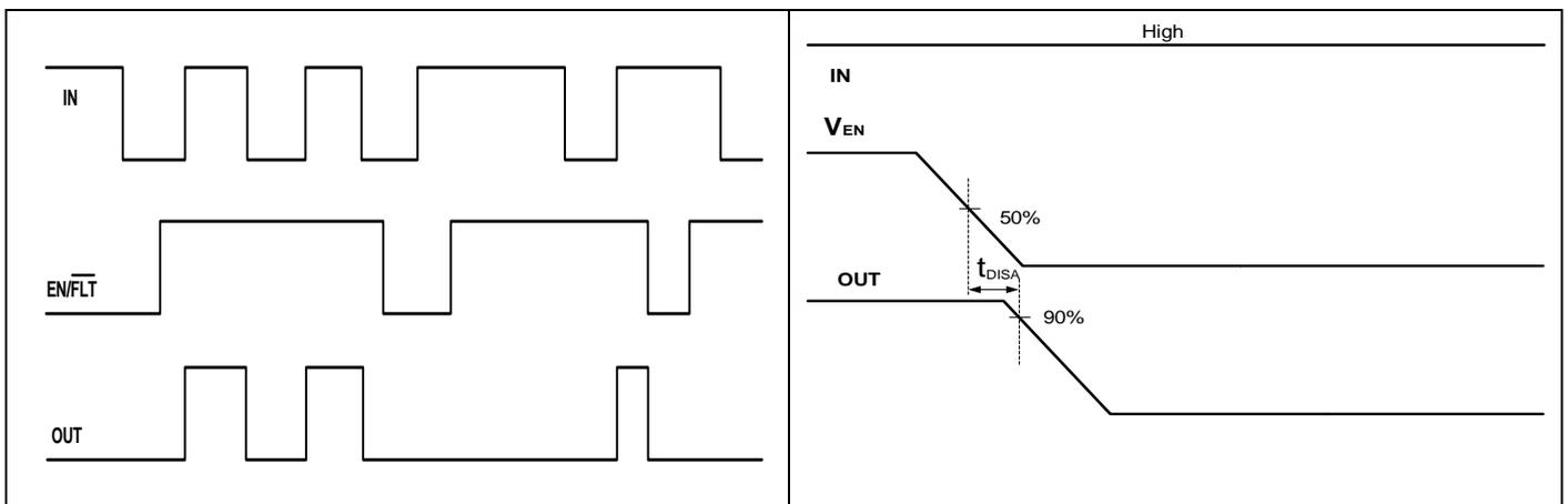
Figure 10 Input/output/enable pins timing diagram Figure 11 EN pin switching time waveform
