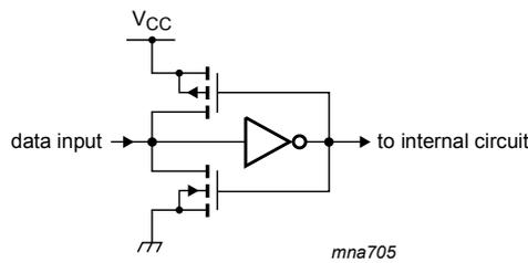
Figure 4. Bus hold circuit
