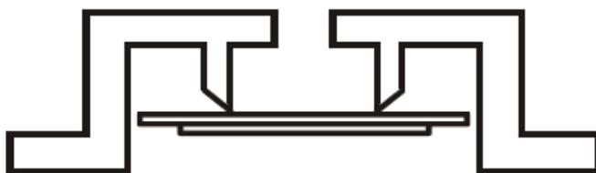
Mounting typically occurs at 60% of the overall diameter of the piezo bender's brass or steel plate. Usually the same diameter as the piezo ceramic element.
