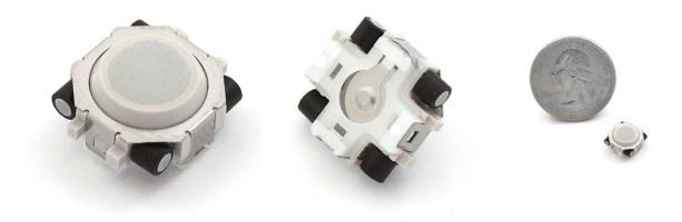
**Description:** This is a tiny trackball akin to those found on a number of Blackberry models (8100, 8300, 8320, 8800, 8830, etc). Each of the four spindles have a tiny circular magnet on each end. Great when paired with very small SMD Hall effect sensors.
