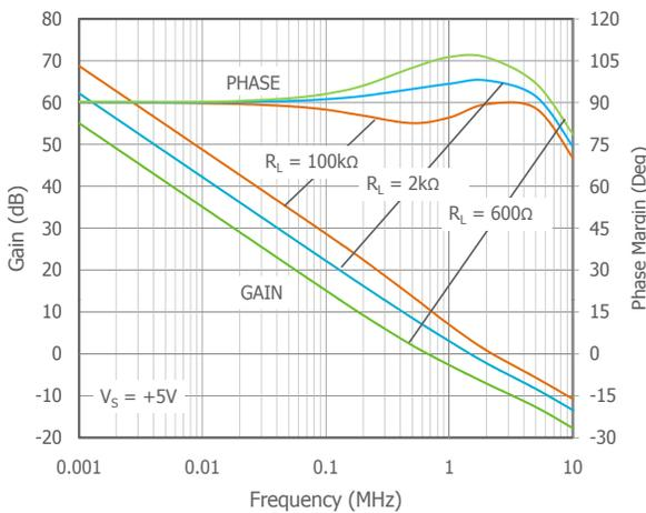
Open Loop Frequency Response vs. Temperature
