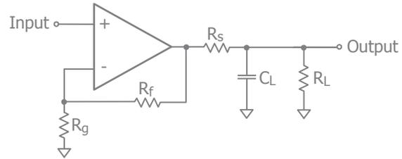
Figure 5. Addition of  $R_S$  for Driving Capacitive Loads
